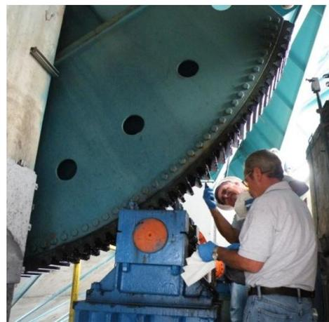
(b) Grease removal from the open gear
