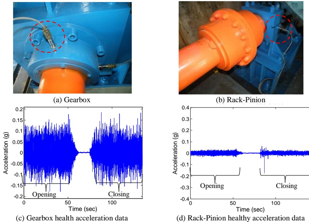
Fig. 5 Sensors on gearbox and rack-pinion with corresponding sample acceleration data
