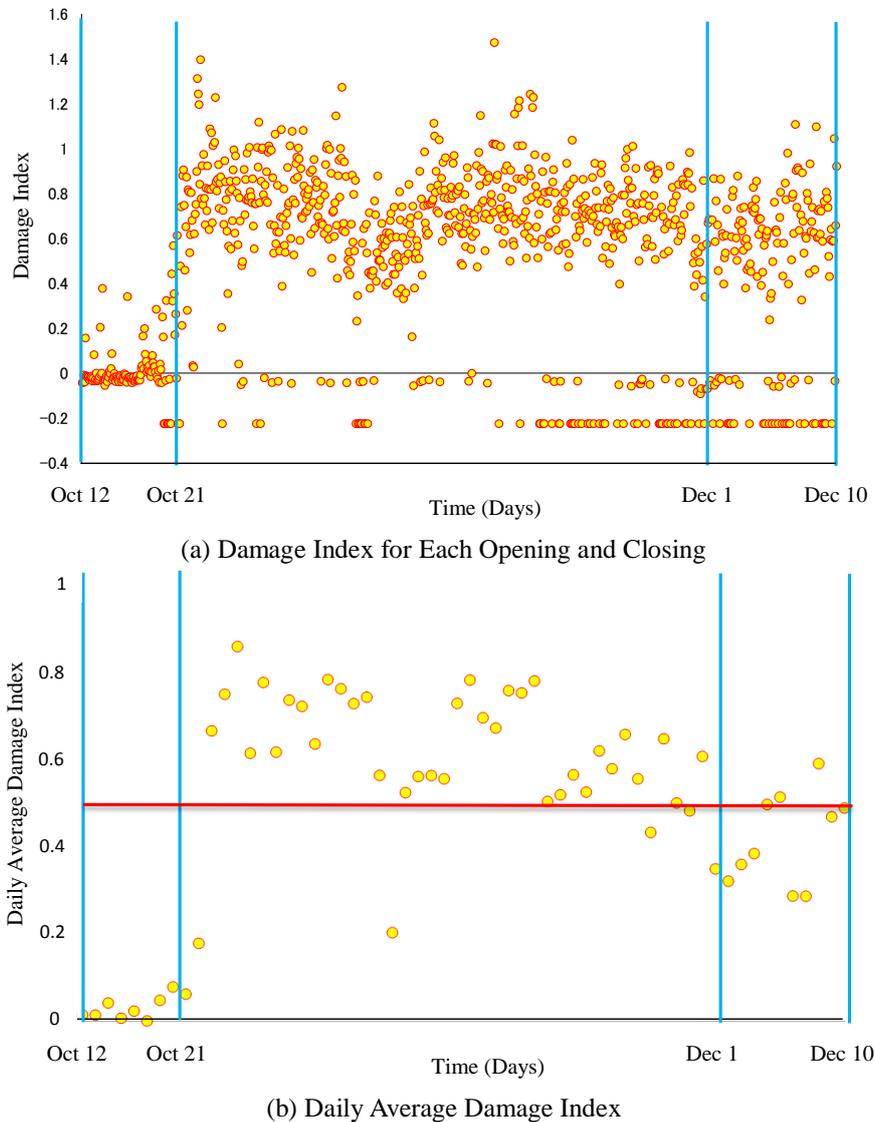
Fig. 12 Monitoring of Rack-Pinion with FNN Model for two Months including Damage (2<sup>nd</sup> Region) and Undamaged Periods (1<sup>st</sup> and 3<sup>rd</sup> Region)
