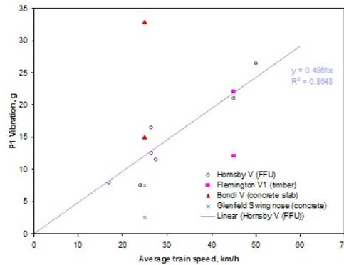
(a) P1 vibration amplitude vs average train speed
