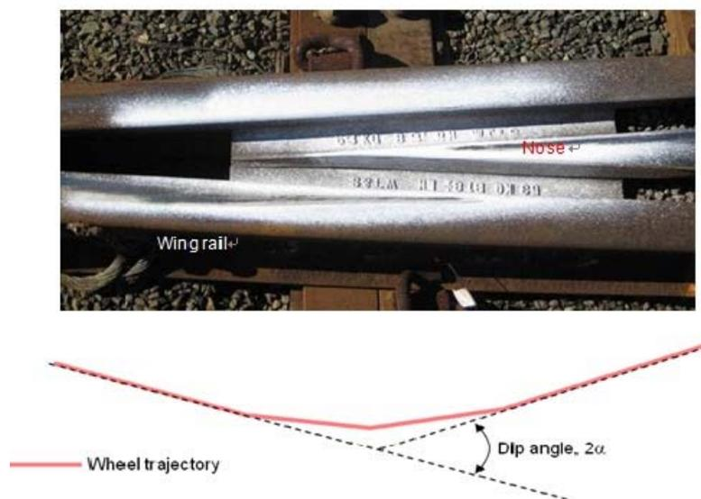
Fig. 2 Transfer zone at crossing where a conical wheel traversing a v-crossing (removal of white paint showing the wheel contact band) and running over a dip angle inducing impact force [1, 2]
