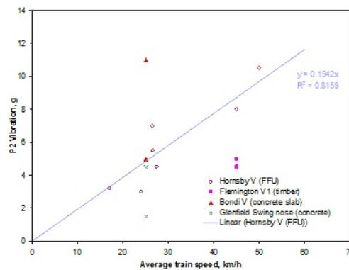
(b) P2 vibration amplitude vs average train speed
