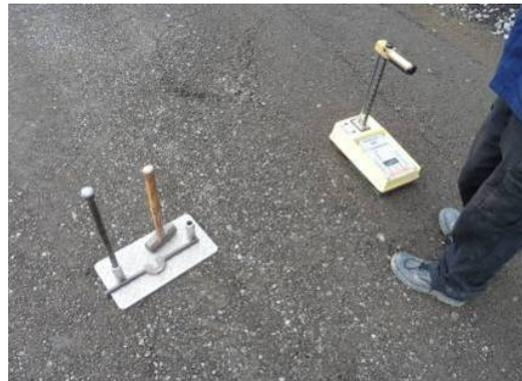
Fig. 8 Compaction test of capping layer
