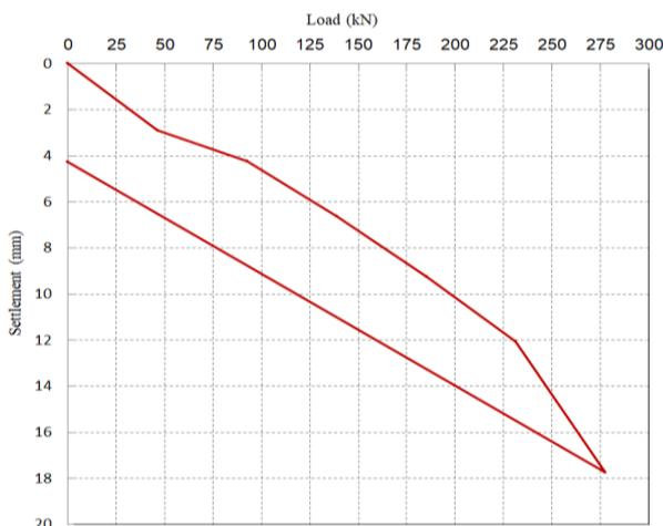
Fig. 7 Relationship between the applied load and the settlement for the tested roof
