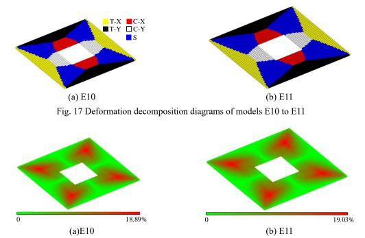
Fig. 18 Warping deformation proportion cloud diagrams of models E10 to E11
