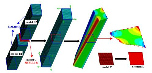
Fig. 8 Schematic diagram of warping deformation of thin plate under torsion condition
