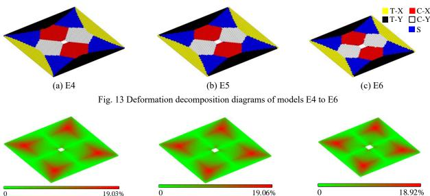
Fig. 14 Warping deformation proportion cloud diagrams of models E4 to E6
