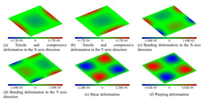
Fig. 6 Deformation cloud diagram of model A1
