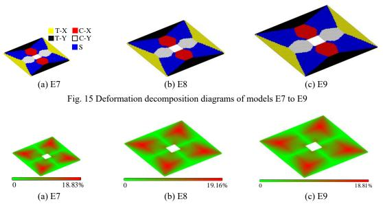
Fig. 16 Warping deformation proportion cloud diagrams of models E7 to E9
