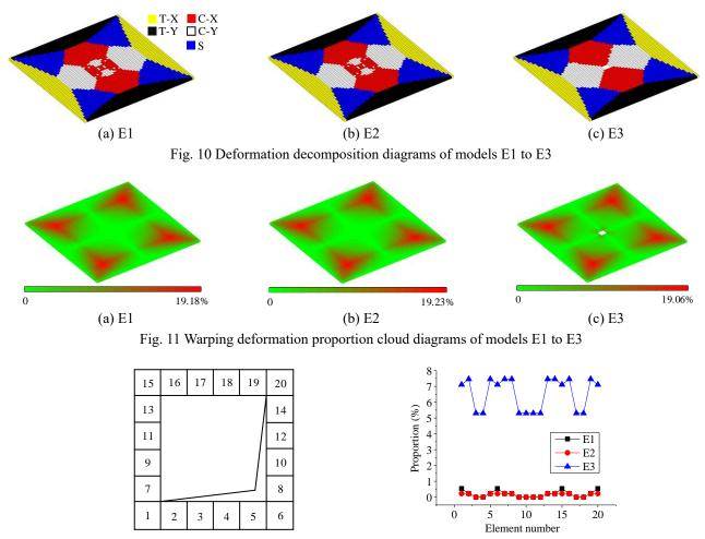
(a) Number of elements around the H-area (b) Proportion of warping deformation of elements
