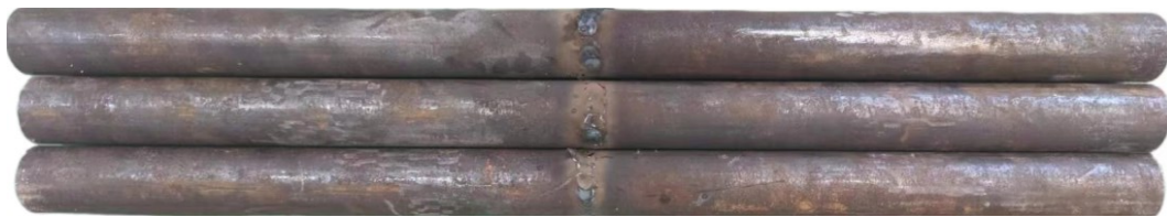
Fig. 2 Seamless steel tubular after welding
