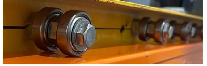
Fig. 4 Arrangement of bearings in the isolation platform
