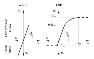
Fig. 6 Stress-strain relationships of concrete
