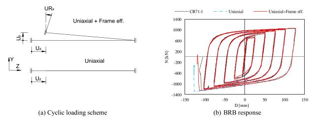
Fig. 23 Influence of the loading scheme on the response of the BRB model
