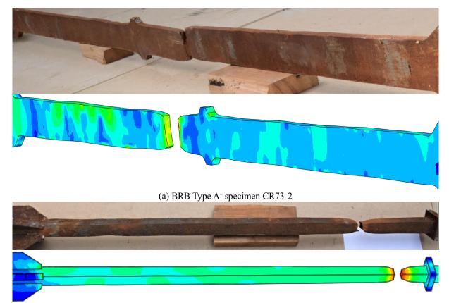
(b) BRB Type B: specimen CS73-2 Fig. 2 Deformed shape of BRB core: experimental vs. FEM
