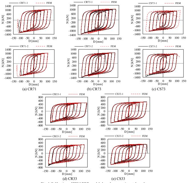
Fig. 1 Calibration of FEM BRB models based on experimental results
