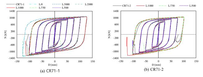
Fig. 9 Effect of initial geometrical imperfections on BRB FEM models CR71
