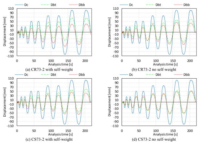
Fig. 22 FEM relative displacements: tube-to-core  $(D_{bt}, D_{bb})$  vs. core end-to-end  $(D_c)$
