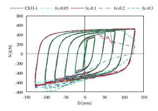
Fig. 3 Calibration of the value of the friction coefficient
