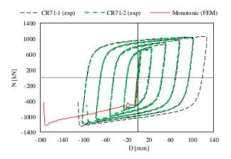
Fig. 14 Calibration of the equivalent imperfection of BRB model under monotonic compression loading
