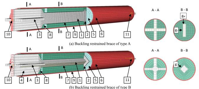
1 - Core: mesh size 10 & 20 mm; C3D8I; steel – combined isotropic-kinematic hardening material.
