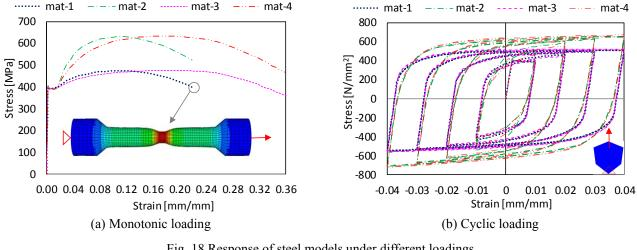
Fig. 18 Response of steel models under different loadings
