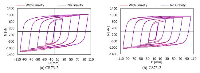
Fig. 21 Influence of self-weight loading on the cyclic response of BRB models
