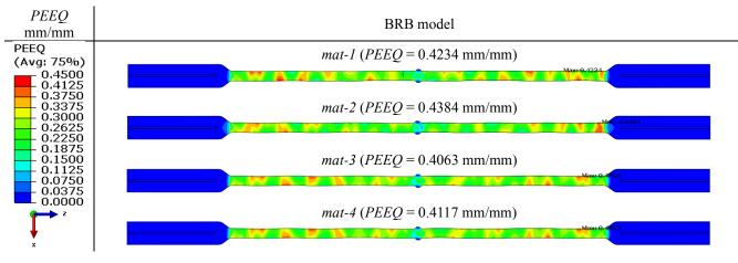
Fig. 20 State of cumulative plastic strain in core at peak compression during the first cycle at  $1.5 D_{bm}$
