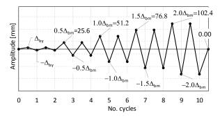
Fig. 13 Loading protocol used for parametric FEM analyses
