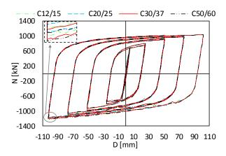
Fig. 17 Cyclic response of BRB models with the concrete infill of different classes
