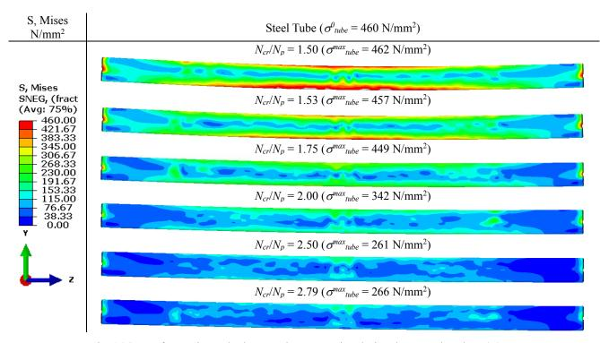
Fig. 16 State of stress in steel tube at peak compression during the second cycle at  $2.0D_{bm}$
