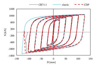
Fig. 7 BRB cyclic predictions using different concrete material models
