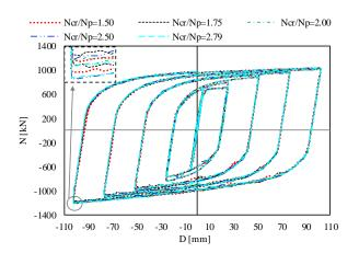
Fig. 15 Cyclic response of BRB models with BRMs of different strength
