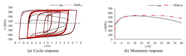
Fig. 4 Calibrated FEM response of core material C30 for the specimens CS33-1 and CR33-2
