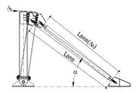
(a) Rigid-body movement of the BRB-column assembly
