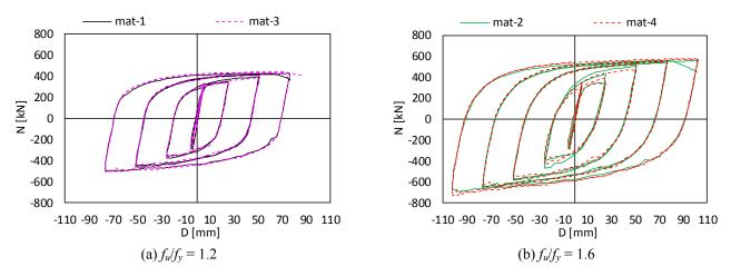
Fig.19 Influence of plastic properties of steel on BRB response under cyclic loading
