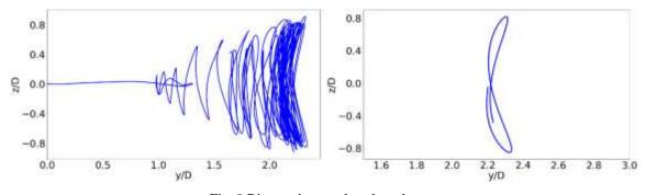
Fig. 9 Riser trajectory, benchmark case
