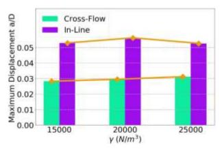
Fig. 24 In-line (left) and cross-flow (right) motions at mudline for different soil unit weight
