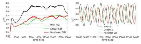
Fig. 16 Comparison of in-line (left) and cross-flow (right) motions, nonlinear SSI
