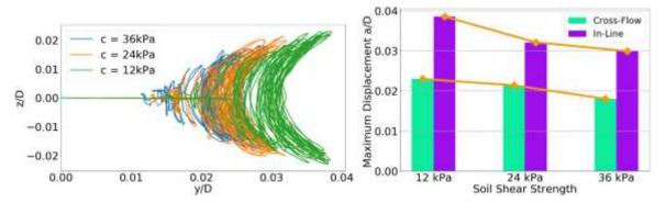
Fig. 22 Trajectories (left) and maximum displacements (right) for different soil strength at mudline
