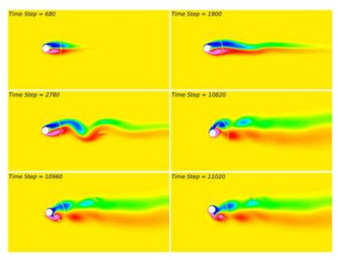
Fig. 15 Vortex generating and shedding, nonlinear SSI
