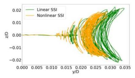
Fig. 19 Trajectories at mudline
