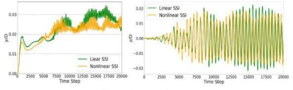
Fig. 18 Comparison of in-line (left) and cross-flow (right) motions at mudline
