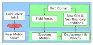
Fig. 2 FSI procedure
