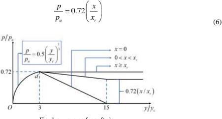
Fig. 1 p-y curves for soft clay
