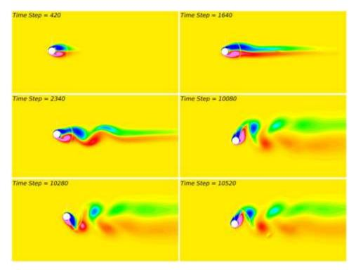
Fig. 6 Vortex generating and shedding, benchmark case
