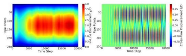
Fig. 10 In-line (left) and cross-flow (right) motion histories, benchmark case
