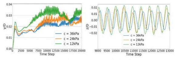
Fig. 21 In-line (left) and cross-flow (right) motions at mudline for different soil strength
