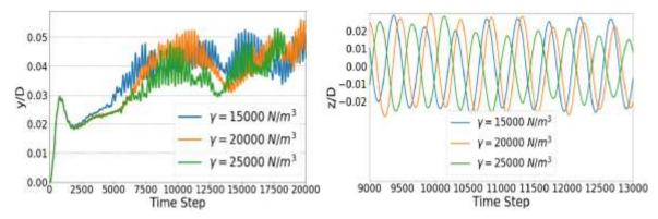
Fig. 23 In-line (left) and cross-flow (right) motions at mudline for different soil unit weight
