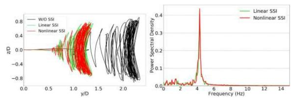
Fig. 17 Comparison of riser trajectories (left) and cross-flow responses, nonlinear SSI
