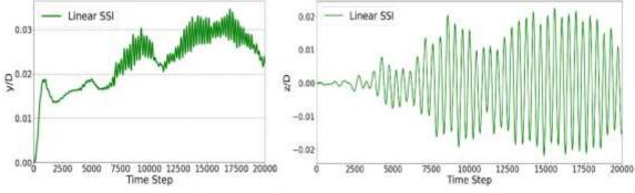
Fig. 14 In-line (left) and cross-flow (right) motion at mudline, simplified SSI
