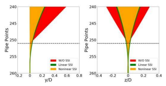
Fig. 20 Comparison of in-line (left) and cross-flow (right) motion envelopes near mudline
