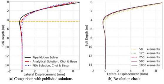
Fig. 5 Validation of SSI model
