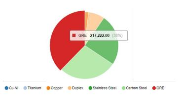
Fig. 4 Rate of materials of pipe at topside
