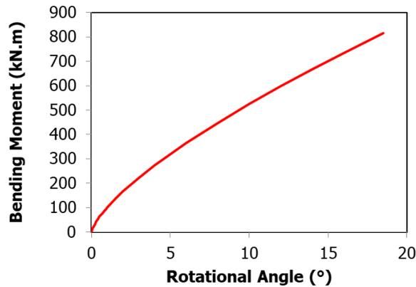
Fig. 6 FlexJoint rotational stiffness
