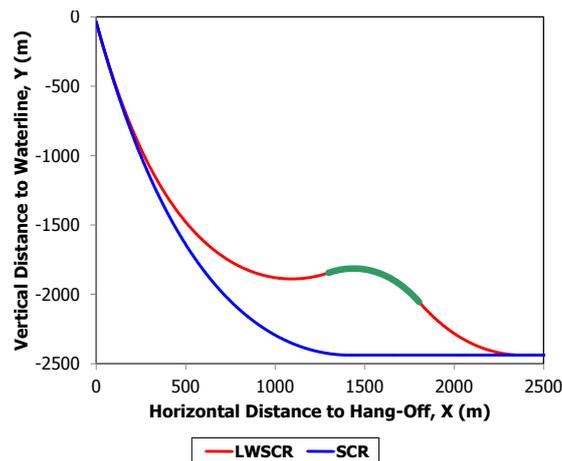
Fig. 7 Base configurations for SCR and LWSCR
