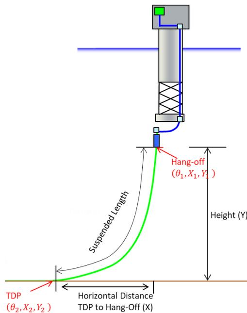
Fig. 2 Typical catenary riser configurations
