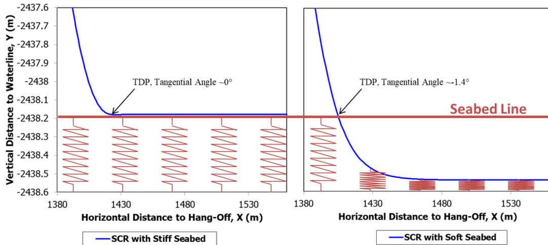
Fig. 5 Pipe-soil interact schematic
