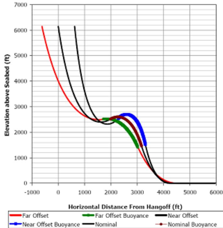
Fig. 4 Variation of lazy wave configuration with vessel offsets (Li and Nyuen 2010)
