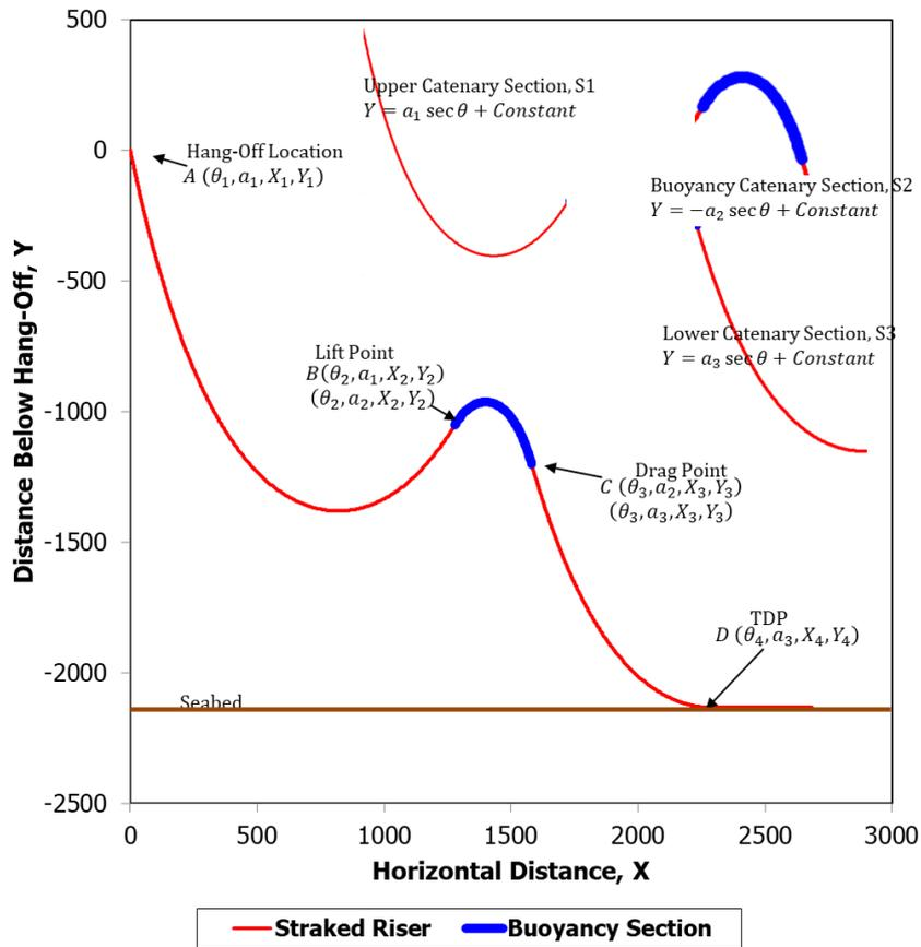
Fig. 3 Typical LWSCR configurations
