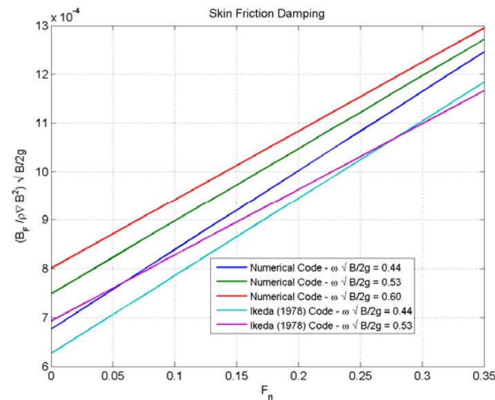
Fig. 6 Forward Speed Skin Friction Damping for Series 60 Hull
