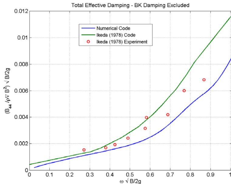
Fig. 1 Zero Speed Total Roll Damping for Series 60 Hull
