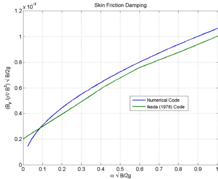
Fig. 5 Zero Speed Skin Friction Damping for a series 60 Hull
