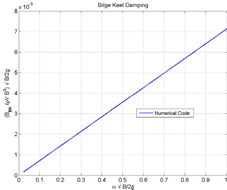
Fig. 10 Zero Speed Bilge Keel Damping for Series 60 Hull
