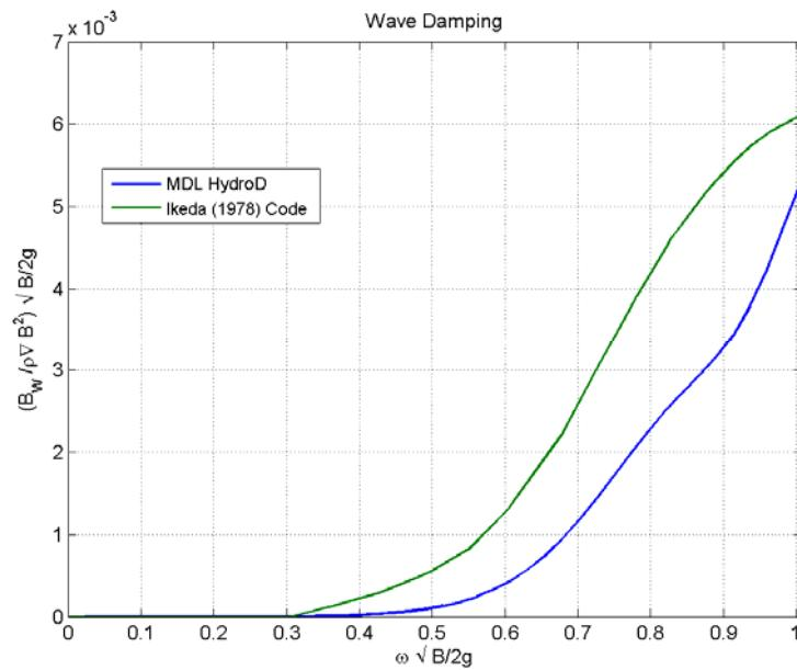
Fig. 3 Zero Speed Wave Damping for Series 60 Hull
