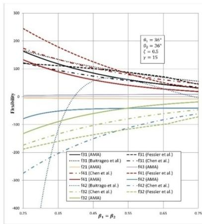
Fig. 16 Effects of  $\beta$  on non-diagonal terms of the LJF matrix for a Symmetric K-joint
