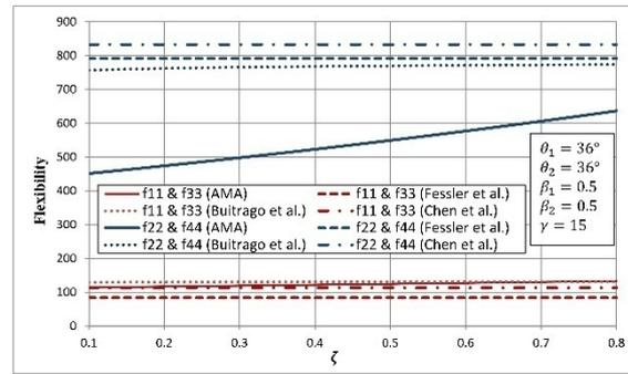
Fig. 9 Effects of  $\zeta$  on main diagonal terms of the LJF matrix for a symmetric K-joint
