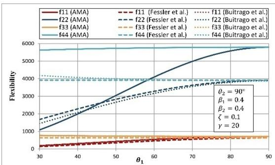
Fig. 12 Effects of  $\theta_1$  on main diagonal terms of the LJF matrix for a Y-T joint
