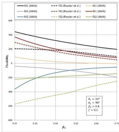
Fig. 20 Effects of  $\beta_1$  on non-diagonal terms of the LJF matrix for a Y-T joint
