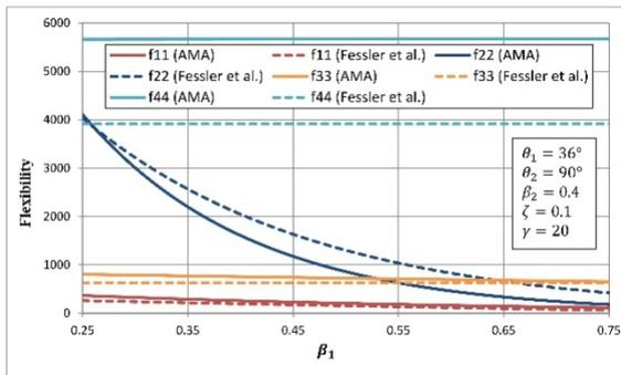
Fig. 10 Effects of  $\beta_1$  on main diagonal terms of the LJF matrix for a Y-T joint
