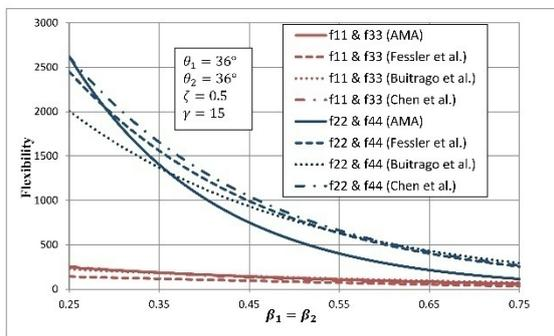
Fig. 6 Effects of  $\beta$  on main diagonal terms of the LJF matrix for a symmetric K-joint
