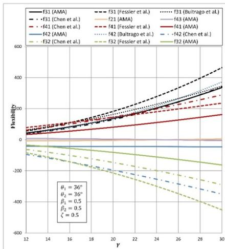
Fig. 18 Effects of  $\gamma$  on non-diagonal terms of the LJF matrix for a Symmetric K-joint
