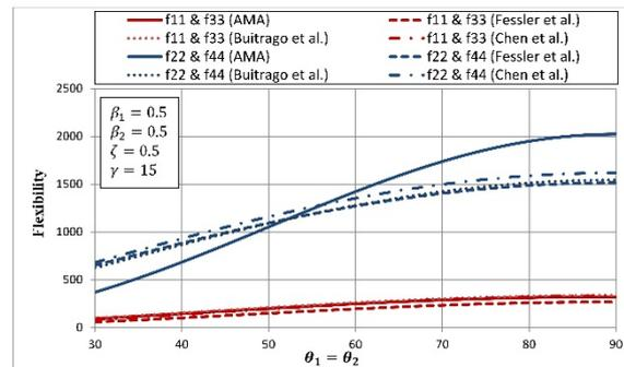
Fig. 7 Effects of  $\theta$  on main diagonal terms of the LJF matrix for a symmetric K-joint
