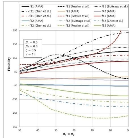
Fig. 17 Effects of  $\theta$  on non-diagonal terms of the LJF matrix for a Symmetric K-joint
