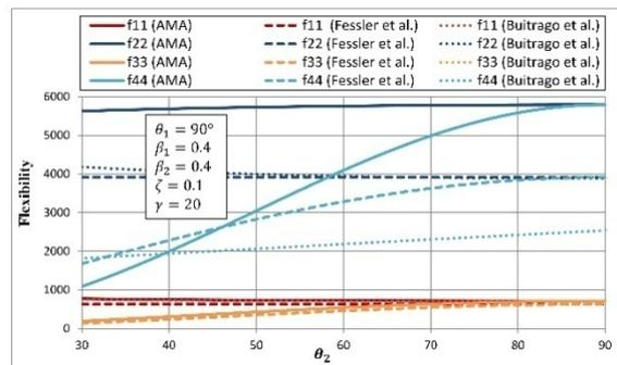
Fig. 13 Effects of  $\theta_2$  on main diagonal terms of the LJF matrix for a Y-T joint
