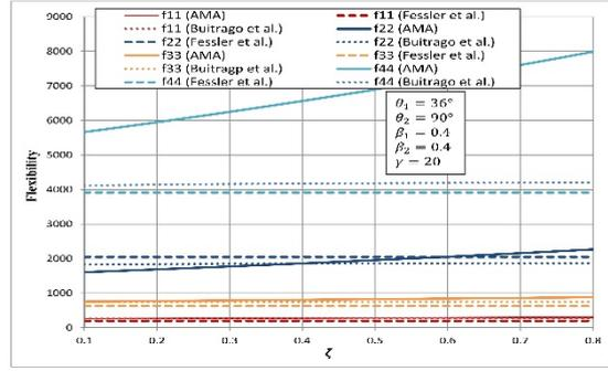
Fig. 15 Effects of  $\zeta$  on main diagonal terms of the LJF matrix for a Y-T joint
