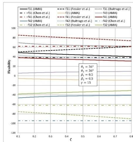
Fig. 19 Effects of  $\zeta$  on non-diagonal terms of the LJF matrix for a Symmetric K-joint
