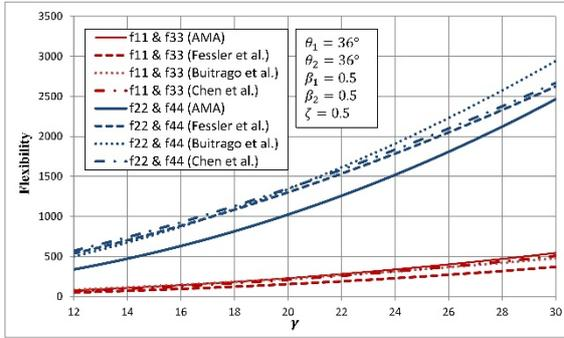
Fig. 8 Effects of  $\gamma$  on main diagonal terms of the LJF matrix for a symmetric K-joint
