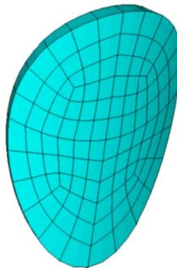
Fig. 3 Mesh generation for the intersection areas between the chord and the braces
