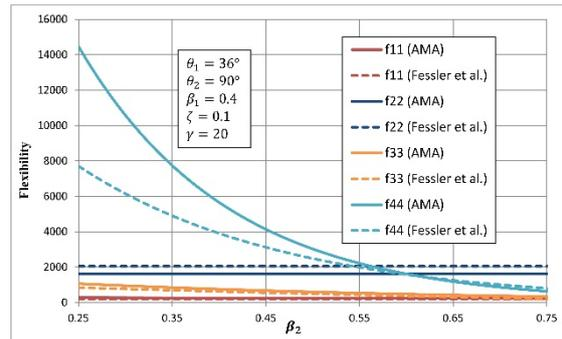
Fig. 11 Effects of  $\beta_2$  on main diagonal terms of the LJF matrix for a Y-T joint
