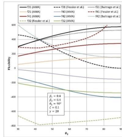
Fig. 23 Effects of  $\theta_2$  on non-diagonal terms of the LJF matrix for a Y-T joint
