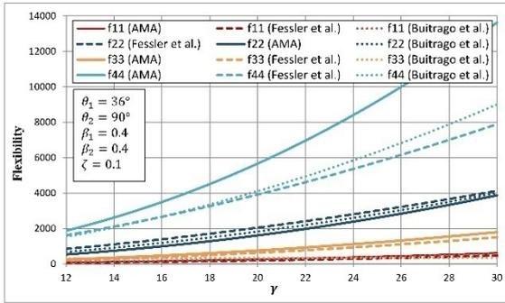
Fig. 14 Effects of  $\gamma$  on main diagonal terms of the LJF matrix for a Y-T joint
