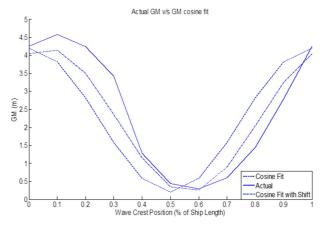
Fig. 6 Comparison of cosine fit of GM with actual GM. (-- Cosine Fit and -.- Cosine Fit with Shift of  $\pi/8$ )
