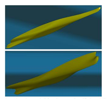
Fig. 4 Change in underwater hull form in waves of modified C11 hull form
