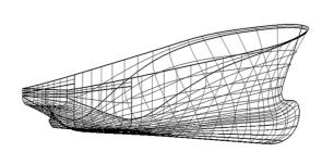
Fig. 2 Body plan of modified C11 hull form (not to scale)
