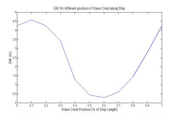
Fig. 5 Variation in GM as the wave crest passes through the hull form
