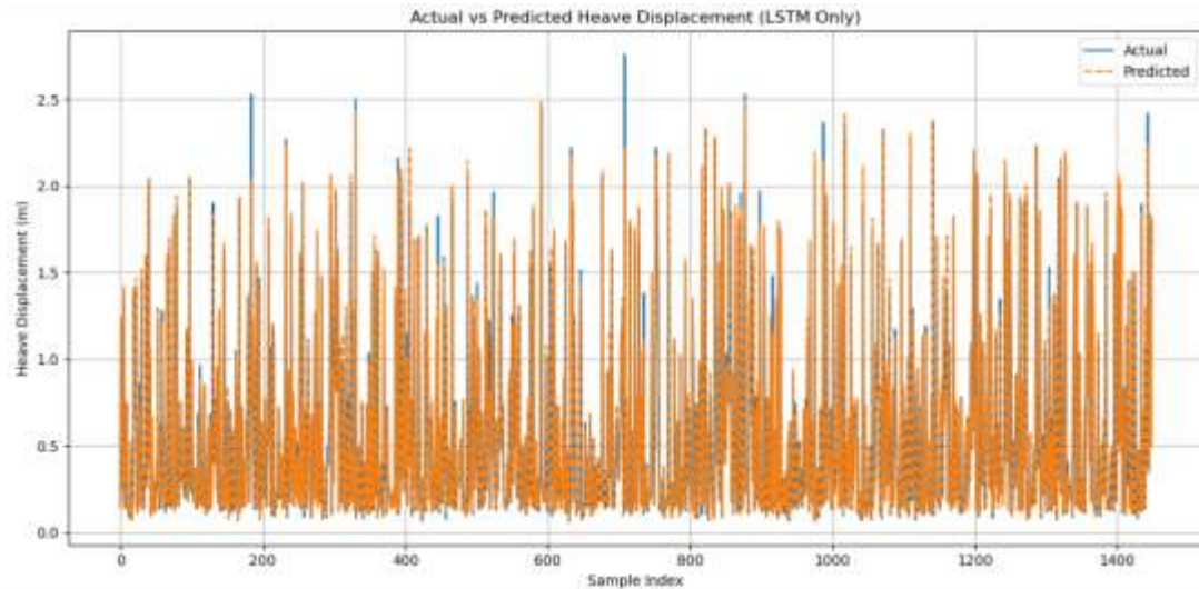
Fig. 7 Actual vs predicted heave displacement for buoy AD06 using the LSTM model
