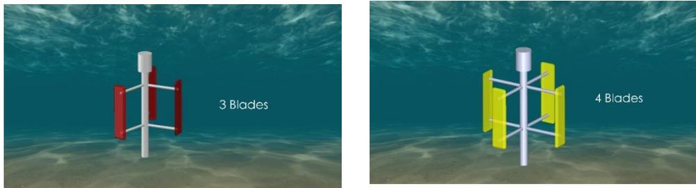
Fig. 2 Vertical Axis Tidal Turbine (a) 4-bladed (b) 3-bladed (Artist impression)
