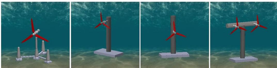
Fig. 1 Examples of Horizontal-Axis Tidal Turbine (a) Piled-Jacket (b) Gravity base (Upper Turbin) (c) Gravity base (Mid Turbin) (d) Monopole-Supported (Artist impression)
