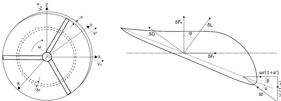
Fig. 5 (a) Disc Model with Blade Element and Regions and (b) Blade Element Velocities and Forces
