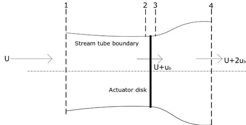
Fig. 4 A visual representation of the Actuator Disk Model
