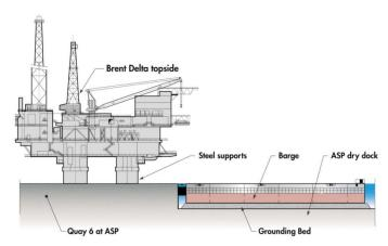
Fig. 3 Topside load-in operation (Shell 2019)
