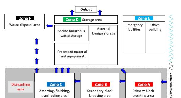
Fig. 5 Layout of ship recycling yard as suggested by UNEP (UNEP 2003)
