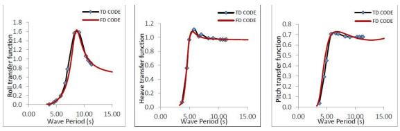
Fig. 7(b) Roll, Heave and Pitch RAOs for 135º heading forward speed condition
