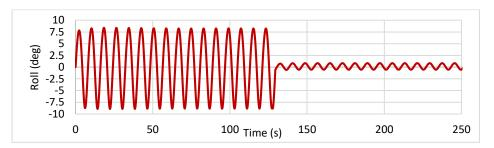
Fig. 13 Controlled and uncontrolled roll motion response at the resonance frequency
