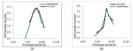
Fig. 9 Roll RAOs for 90° heading for zero speed (a) and forward speed (b) condition
