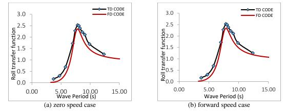
Fig. 6 Roll RAOs for 90° heading for zero speed (a) and forward speed (b) condition
