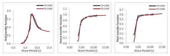
Fig. 7(b) Roll, Heave and Pitch RAOs for 135º heading zero speed condition
