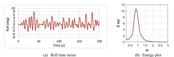
Fig. 17 Roll motion time series and energy plot for vessel subjected to Sea State 4 for 135° wave heading
