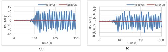
Fig. 15(a) Parametric Roll Stabilization with fin control for  $180^{\circ}$  heading and (b) Parametric Roll Stabilization with fin control for  $170^{\circ}$  heading
