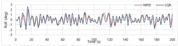
Fig. 20 Roll motion response comparison for NPID and LQR controller for the vessel in Sea State 4 and 90° wave heading
