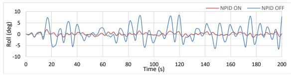
Fig. 19 Controlled and uncontrolled roll motion response for ship subjected to irregular waves at Sea State 4 and  $90^{\circ}$  wave heading.
