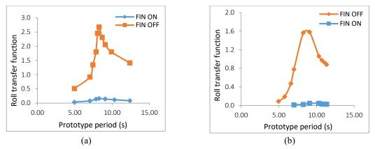
Fig. 14(a) Roll RAO for 90° heading and (b) Roll RAO for 135° heading
