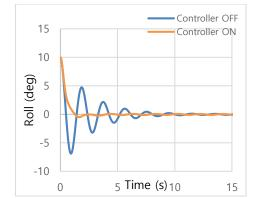
Fig. 3 Roll decay response for the vessel with and without control action
