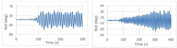
(a) wave length/ship length =1 (b) wave length/ship length =1.2 Fig. 10 Parametric Rolling identified in vessel subjected to wave steepness = 1/12 and 180° heading
