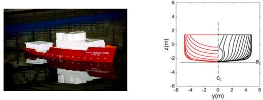
Fig. 5 The fabricated model and the body plan of the vessel (Subramanian et al. 2020)
