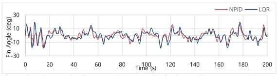
Fig. 21 Fin angle comparison for NPID and LQR controller for the vessel in Sea State 4 and 90° wave heading
