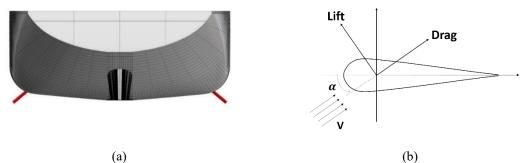
Fig. 2 Typical arrangement of the fins (a) and schematic of fin forces (b)
