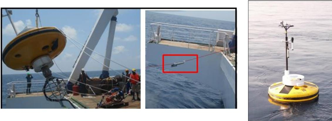
Fig. 2 OMNI buoy being deployed from ORV Sagar Kanya, Venkatesan (2013,2016, 2017)
