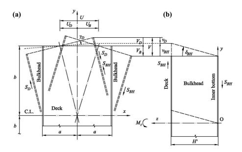
Fig. 6 Deck and bulkhead displacements and in-plane deformations, (a) bird's eye view on the deck, (b) axial view on the transverse bulkhead.
