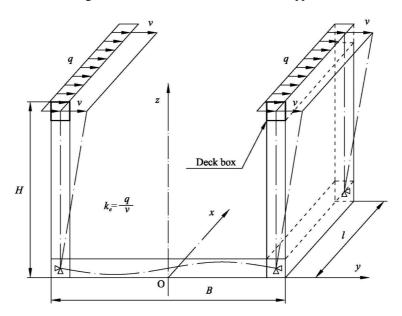
Fig. 8 Definition of deck box support stiffness
