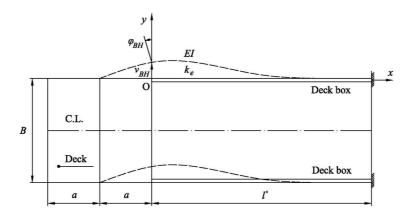
Fig. 7 Deck boxes as beams on elastic supports
