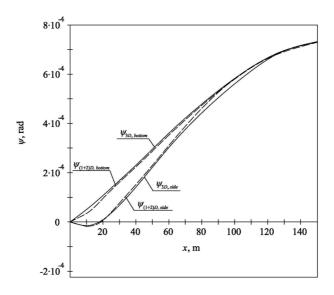
Fig. 16 Twist angles of segmented pontoon
