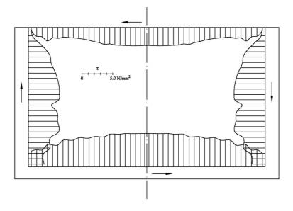
Fig. 15 Shear stresses at internal boundary of front engine room bulkhead
