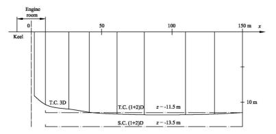
Fig. 18 Vertical position of twist centre
