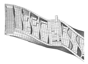
Fig. 1 Bird's eye view of the 7800 TEU container ship aftbody, the 2<sup>nd</sup> natural mode
