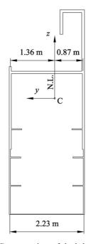
Fig. 11 Cross-section of deck box girders
