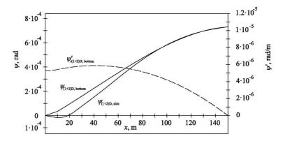
Fig. 10 Deformation functions of segmented pontoon
