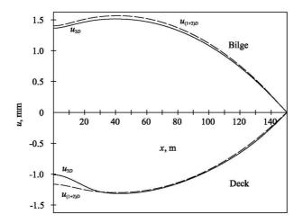
Fig. 17 Axial displacements of deck and bottom
