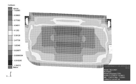
Fig. 14 Shear stresses in front engine room bulkhead
