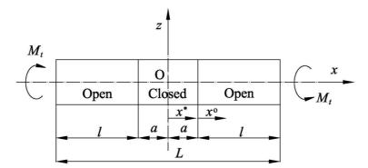
Fig. 9 Torsion of segmented girder
