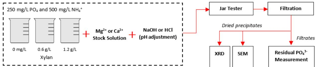
Fig. 2 Schematic diagram for xylan experiment on struvite and hydroxyapatite precipitation
