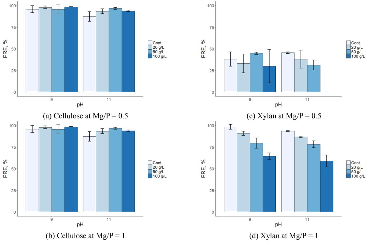
Fig. 3 Effect of different amounts of cellulose and xylan on phosphorus removal at varying Mg/P molar ratios
