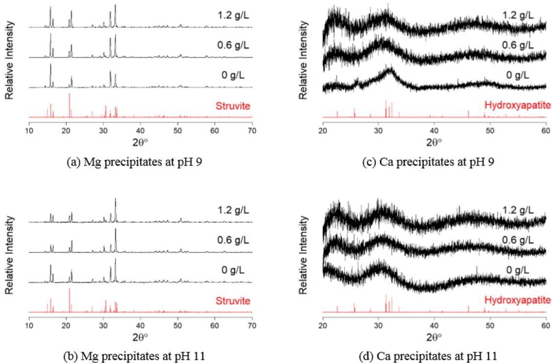
Fig. 6 XRD patterns for Mg and Ca precipitates at varying pH and xylan concentrations along with reference pattern
