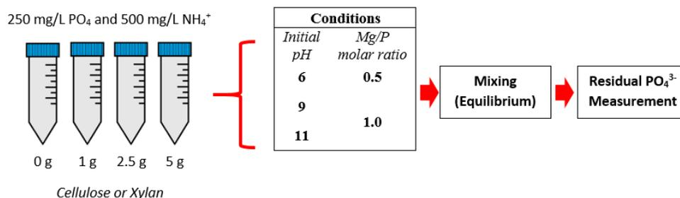
Fig. 1 Schematic diagram for cellulose and xylan experiment
