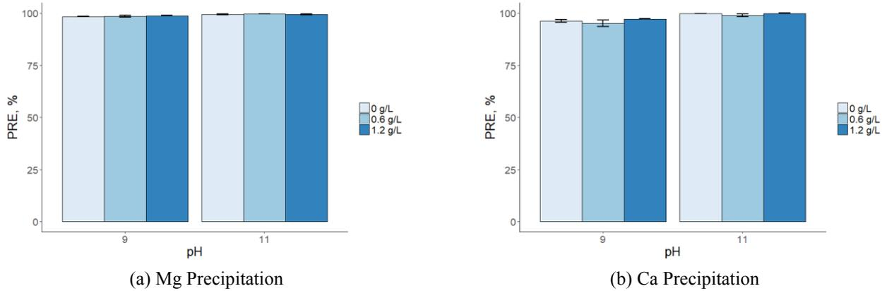
Fig. 4 Phosphorus removal rates for Mg and Ca precipitation at varying xylan concentration, and pH at 1.5 Mg/P and 2.5 Ca/P molar ratios
