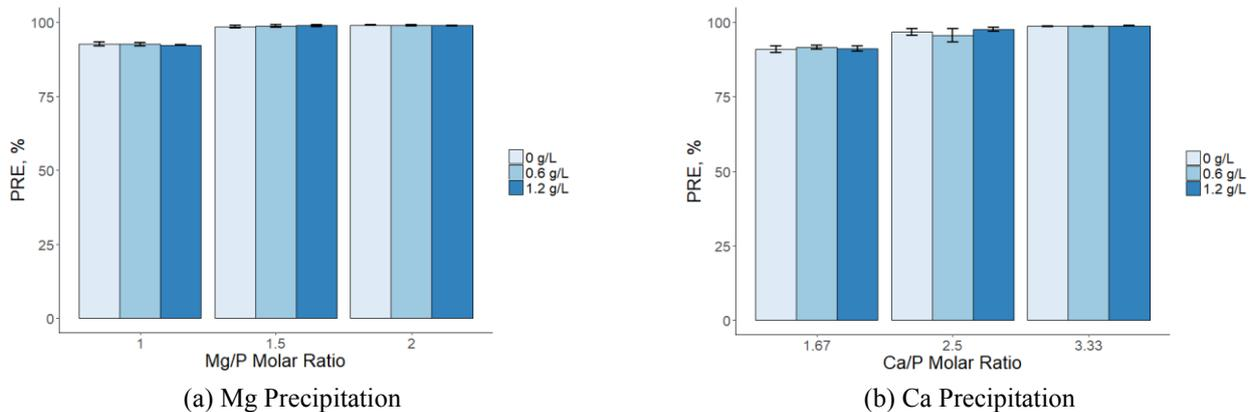
Fig. 5 Phosphorus removal rates for Mg and Ca precipitation at varying xylan concentration and molar ratios at pH 9
