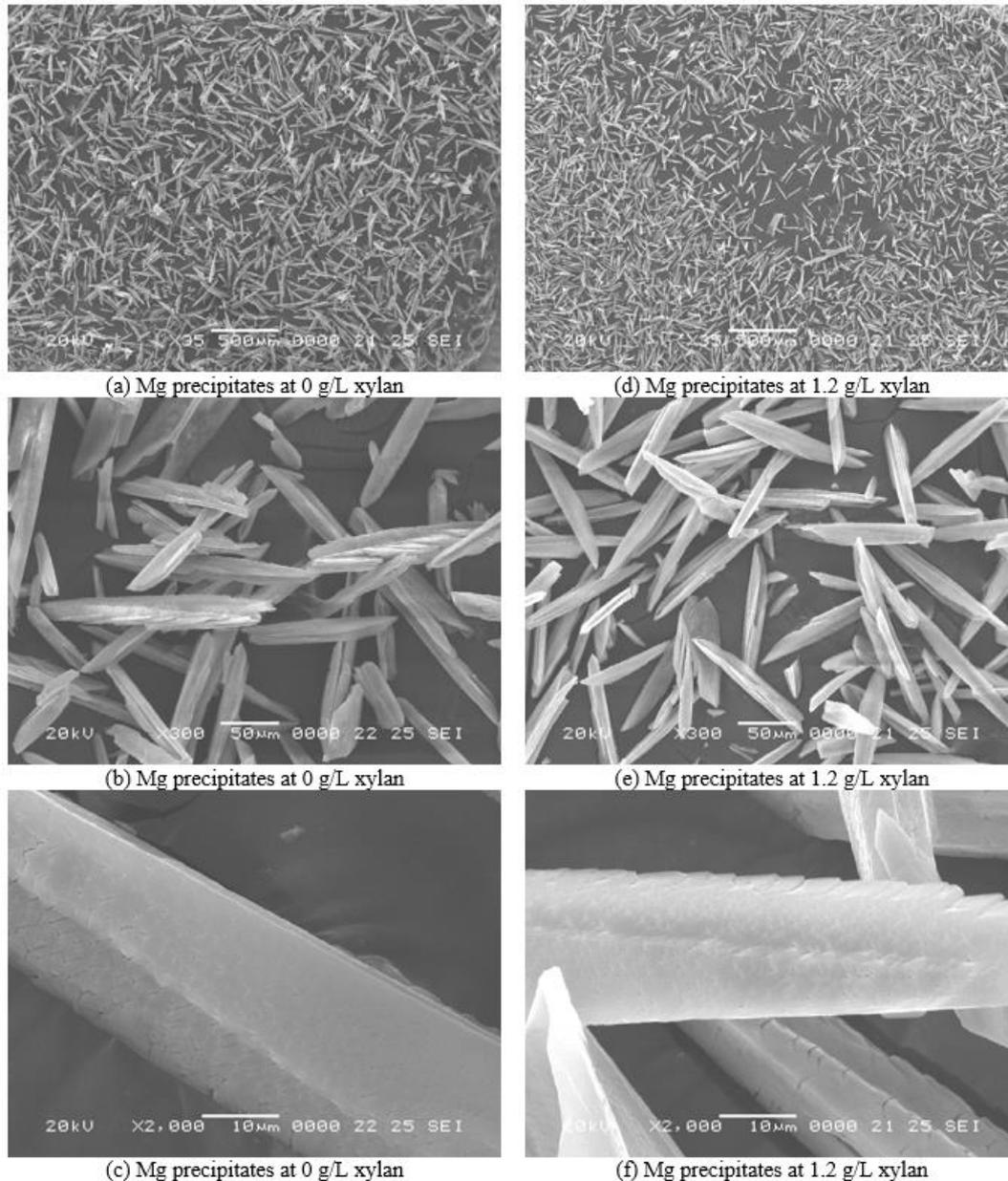
Fig. 7 SEM images of Mg precipitates at (a)-(c) 0 g/L and (d)-(f) 1.2 g/L xylan concentration at different magnifications
