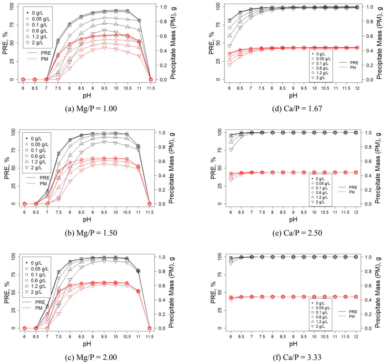
Fig. 9 MINTEQ model of the effect of HS on phosphorus removal by addition of (a)-(c) Mg and (d)-(f) Ca.
