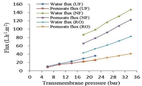
Fig. 2 Effect of transmembrane pressure on permeate flux for clean water and natural rubber wastewater
