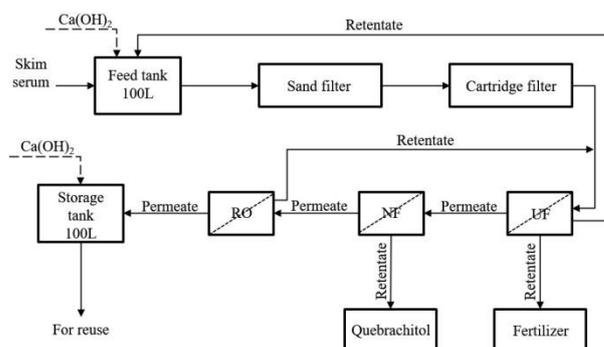
Fig. 1 Schematic diagram of the laboratory scale membrane system
