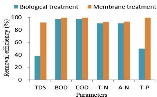
Fig. 5 Comparison of the membrane and biological systems for removal efficiency of respective parameters
