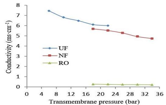
Fig. 3 Effect of transmembrane pressure on conductivity in the membrane experiments
