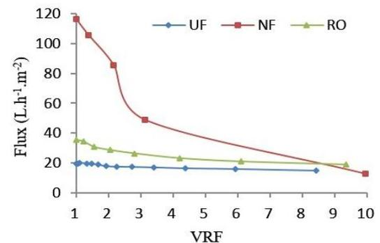
Fig. 4 Effect of the volume reduction factor on permeate flux in the membrane experiments
