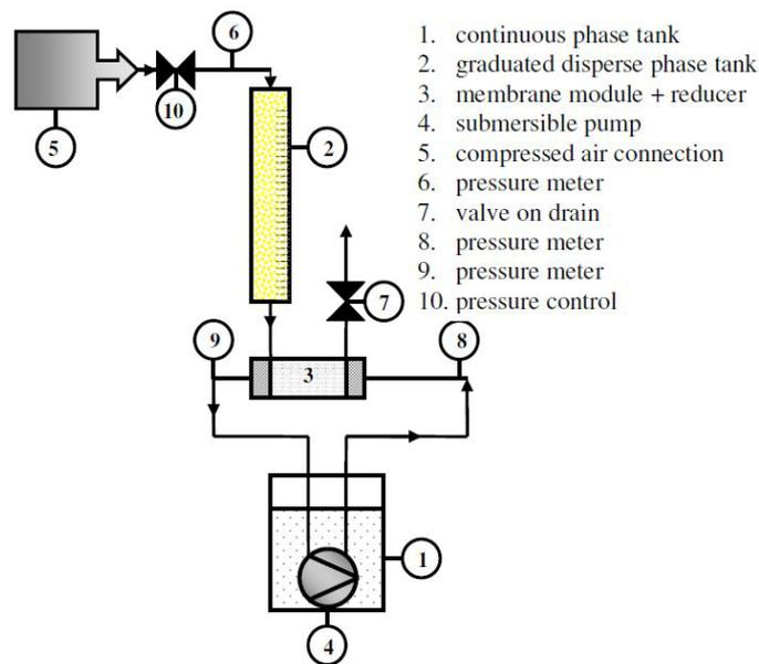
Fig. 1 Scheme of the cross-flow membrane emulsification apparatus
