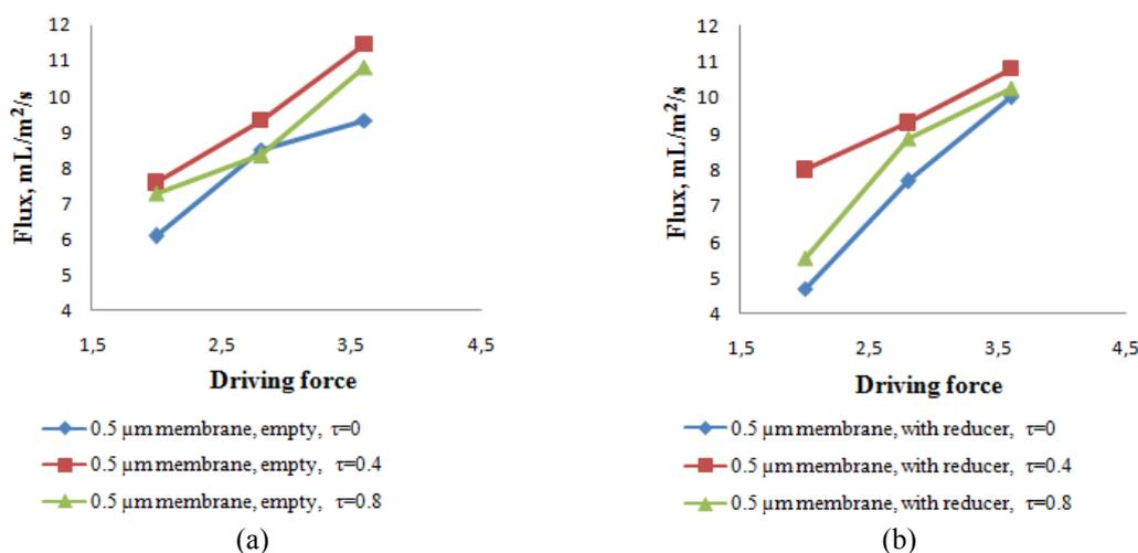
Fig. 3 Dispersed phase flux values on different driving forces and shear-stresses (a) without reducer; and (b) with reducer
