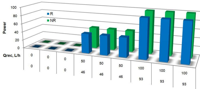
Fig. 10 Relative pumping energy consumption to recycle the continuous phase
