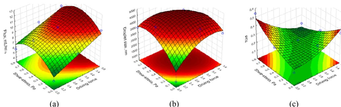
Fig. 9 Fitted 3D surfaces the effects of driving force and shear-stress on (a) flux; (b) droplet size; and (c) PDI in case of using reducer, 0.5  $\mu\text{m}$  membrane
