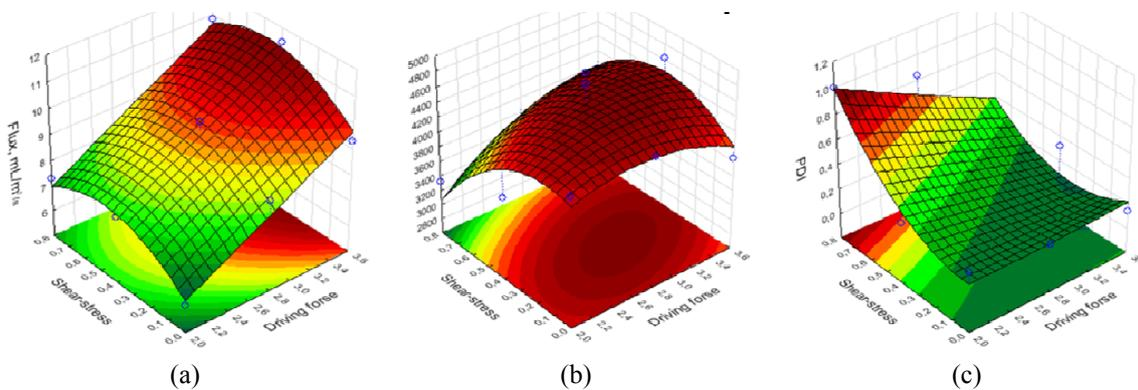
Fig. 8 Fitted 3D surfaces the effects of driving force and shear-stress on (a) flux; (b) droplet size; and (c) PDI in case of empty tube, 0.5  $\mu\text{m}$  membrane
