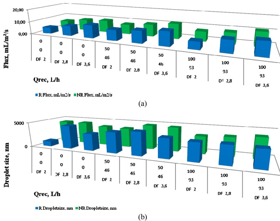
Fig. 4 (a) Difference of flux; (b) droplet size; and (c) PDI with or without reducer for 0.5 μm membrane
