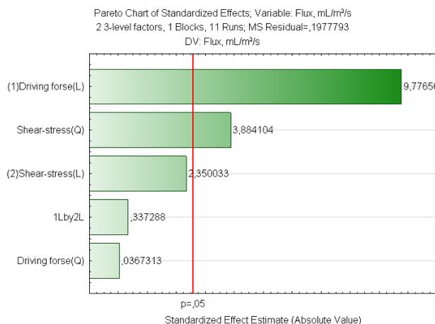
Fig. 7 Pareto chart of standardized effect on flux (0.5  $\mu\text{m}$ , without reducer)
