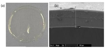
Fig. 1 Aliquat/PVC polymer inclusion membranes: (a) a real scale image of the membrane and (b) an SEM micrograph of the membrane cross section
