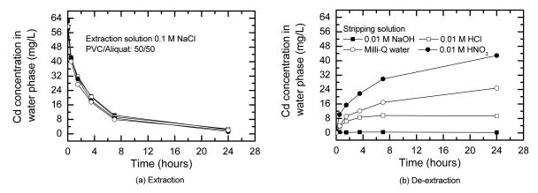
Fig. 4 (a) Extraction and (b) de-extraction (stripping) kinentics of cadmium to PVC/Aliquat PIMs (wt/wt = 50%/50%)
