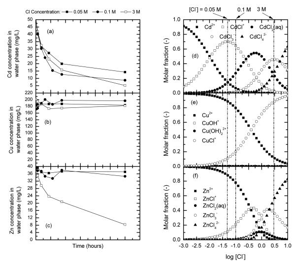
Fig. 3 Extraction of (a) Cd(II), (b) Cu(II), and (c) Zn(II) into PVC/Aliquat PIMs (wt/wt = 50%/50%) from solutions containing different NaCl concentration. The speciation of (d) cadmium, (e) cupper, and (f) zinc chloro complex as a function of NaCl concentration (solution chemistry is the same as the extraction experiments)
