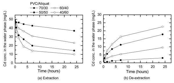
Fig. 2 (a) Extraction and (b) de-extraction (stripping) kinentics of cadmium to PIMs with different PVC and Aliquat 336 contents. Extraction solution contained 50 mg/L Cd in 0.05 M NaCl solution. Milli-Q water was used as the stripping solution
