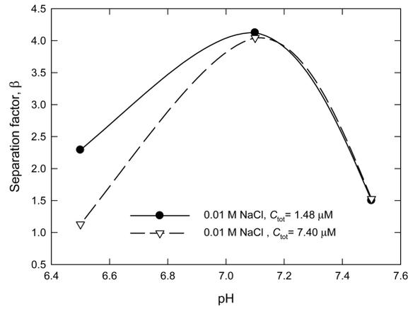
Fig. 8 Effect of pH on the separation factor in the presence of 0.01 M NaCl under different total protein concentrations
