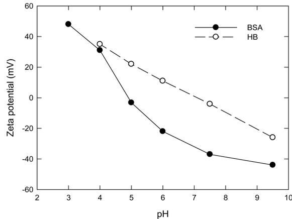
Fig. 2 Zeta potentials of BSA and HB at different pH values
