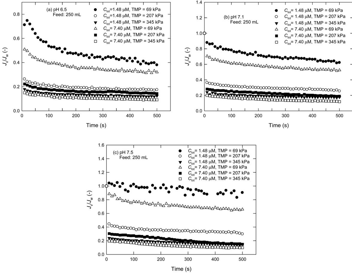
Fig. 3 Time changes of normalized flux at the pH value of (a) 6.5, (b) 7.1, and (c) 7.5
