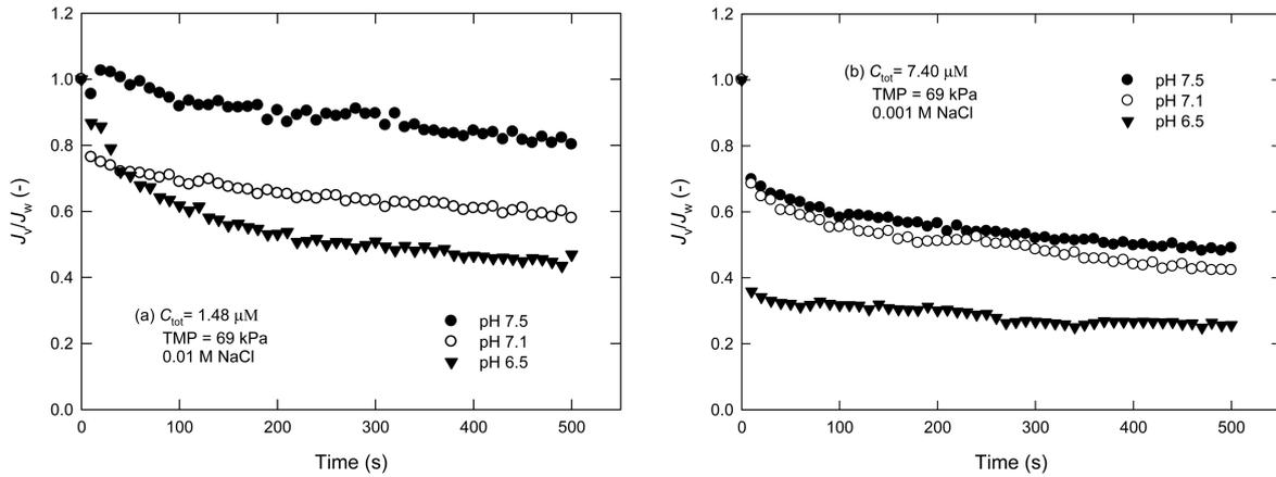
Fig. 7 Time changes of normalized flux in the presence of 0.01 M NaCl at the total protein concentration of (a) 1.48 and (b) 7.40  $\mu\text{M}$
