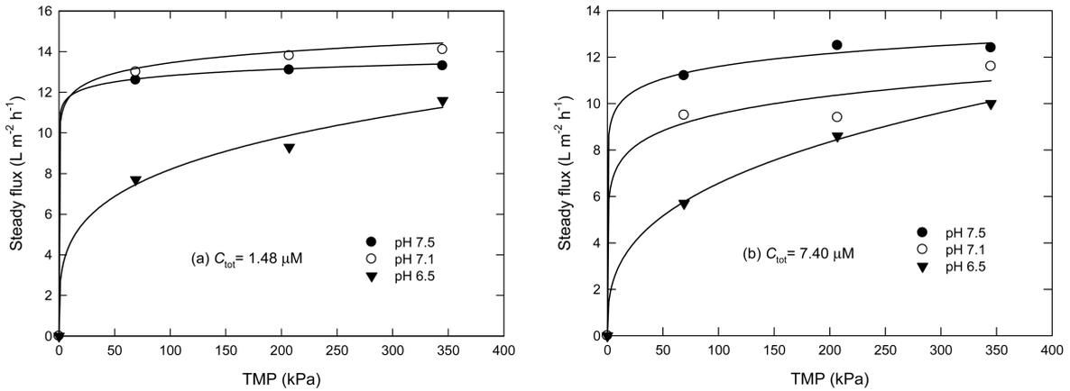
Fig. 4 Effect of TMP on steady-state flux at the total protein concentration of (a) 1.48 and (b) 7.40  $\mu\text{M}$
