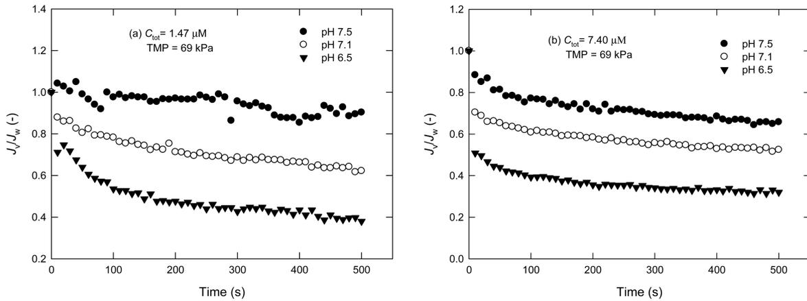
Fig. 6 Time changes of normalized flux in the absence of NaCl at the total protein concentration of (a) 1.48 and (b) 7.40  $\mu\text{M}$
