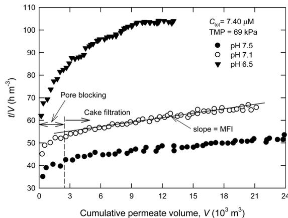
Fig. 9 Typical plot for the determination of modified fouling index (MFI) in the present UF process
