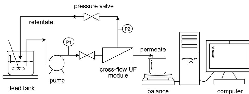
Fig. 1 Schematic diagram of the experimental setup involving cross-flow UF system
