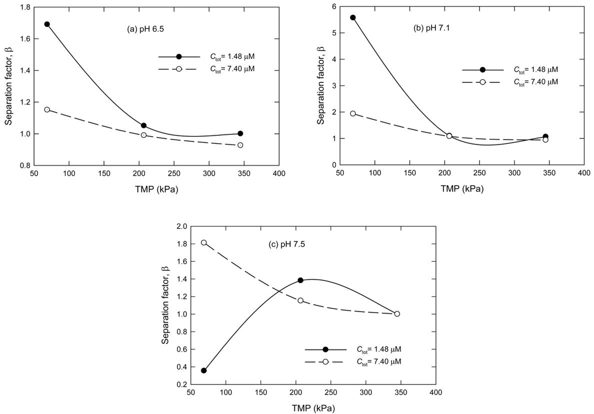
Fig. 5 Effect of TMP on separation factor at the pH value of (a) 6.5, (b) 7.1, and (c) 7.5
