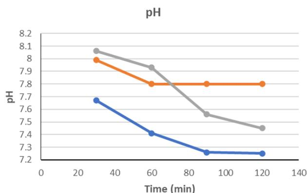
Fig. 2 pH values using different adsorbent doses at different contact times
