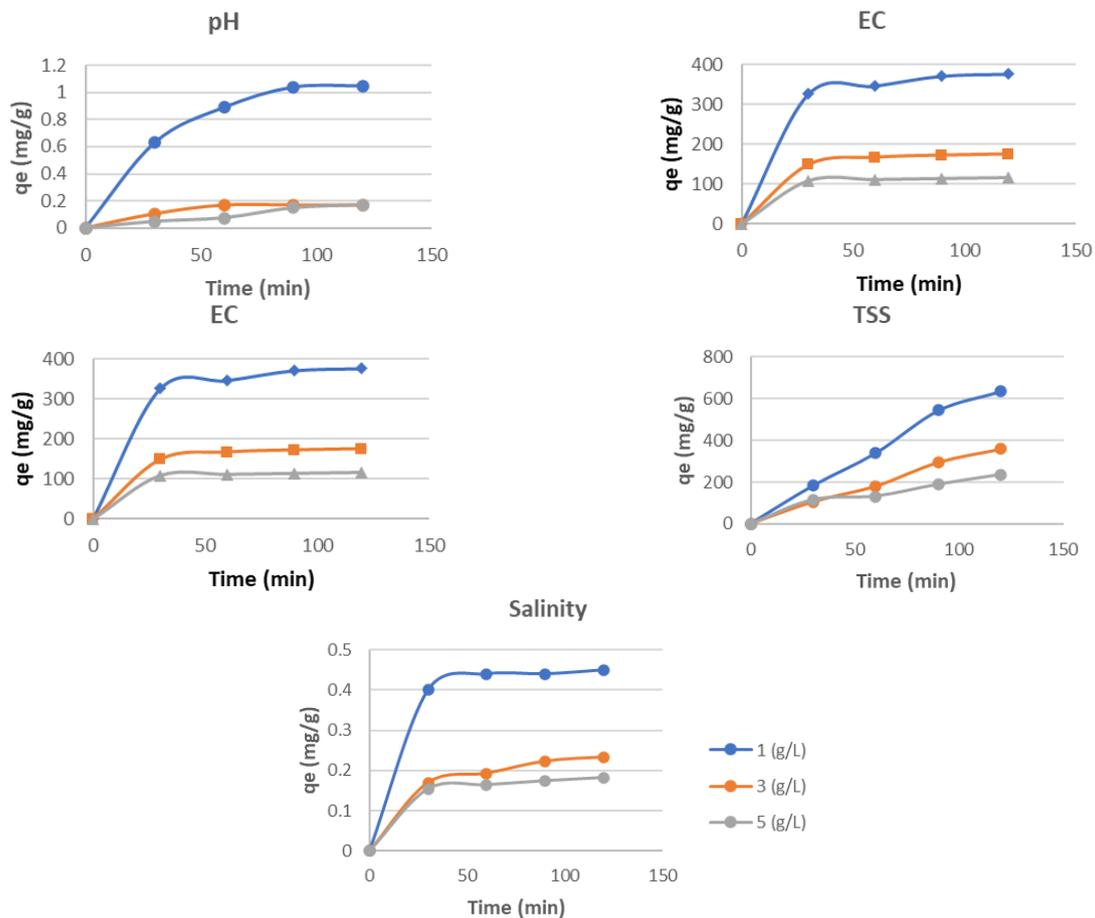
Fig. 4 Adsorption profile of pH, EC, TDS, TSS and salinity values using different adsorbent doses at different contact times
