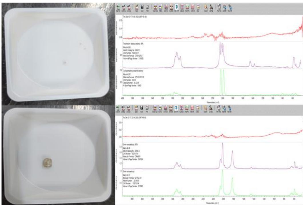
Fig. 6 Sample qualitative analysis results of micro-plastic based on FT-IR
