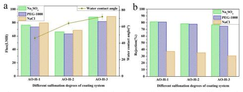
Fig. 5 (a) The flux, water contact angle and (b) Rejection of composite membrane with different sulfonation degrees of coating system
