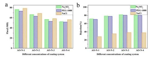
Fig. 6 (a) The flux and (b) Rejection of composite membrane with different concentrations of coating system
