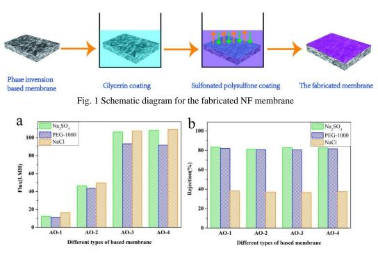
Fig. 2 (a) The flux and (b) Rejection of composite membrane with different types of based membrane
