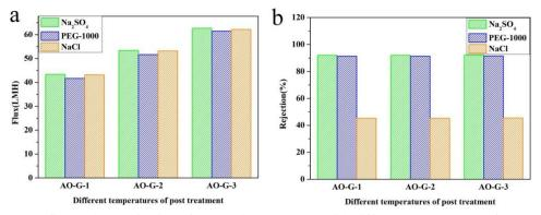
Fig. 9 (a) The flux and (b) Rejection of composite membrane with different temperatures of post treatment
