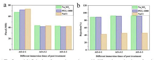
Fig. 8 (a) The flux and (b) Rejection of composite membrane with different immersion times of coating system
