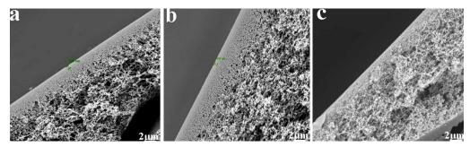
Fig. 10 SEM images of the different temperatures of post treatment progress. (a) nature wind; (b) low temperature air knife; (c) high and low temperature variable frequency air knife
