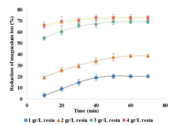
Fig. 10 The reduction of magnesium ion versus contact time using Amberlite IR120 H<sup>+</sup> at 25°C and 350 rpm
