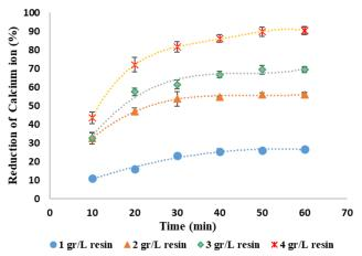
Fig. 9 The reduction of calcium ion versus contact time using Amberlite IR120  $H^+$  at 25°C and 350 rpm
