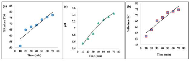
Fig. 20 The reduction of (a) TDS, (b) EC and (c) pH at optimum concentration, (3 g/L cationic resin and 12 g/L anionic resin)
