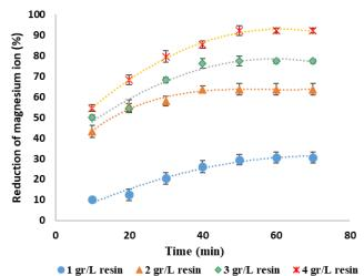
Fig. 4 The reduction of magnesium ion versus contact time using Purolite C-100 Na<sup>+</sup> at 25°C and 350 rpm
