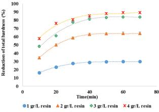
Fig. 5 The reduction of total hardness versus contact time using Ambersep IR252  $H^+$  at 25°C and 350 rpm
