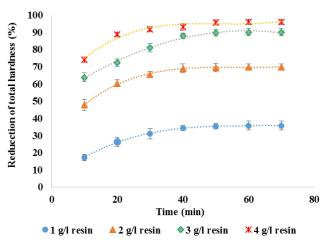
Fig. 2 The reduction of total hardness versus contact time using Purolite C-100 Na<sup>+</sup> at  $25^{\circ}$ C and 350 rpm
