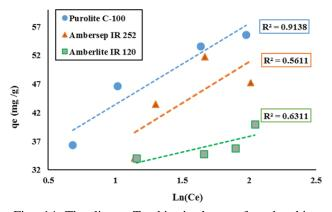
Fig. 14 The linear Temkin isotherms for absorbing calcium ion using Purolite C-100 Na<sup>+</sup>, Ambersep IR 252 H<sup>+</sup> and Amberlite IR 120 H<sup>+</sup>, under experimental condition of constant initial concentration, 60 min contact time, 350 rpm and  $25^{\circ}$ C
