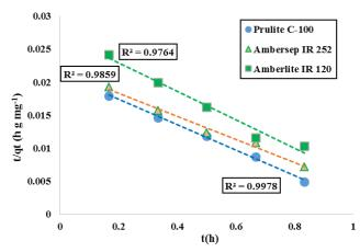
Fig. 17 The linear pseudo-second-order kinetic model for absorbing calcium ion using Purolite C-100 Na<sup>+</sup>, Ambersep IR 252 H<sup>+</sup> and Amberlite IR 120 H<sup>+</sup> under the experimental condition of constant initial concentration, 60 min contact time, 350 rpm, and  $25^{\circ}$ C
