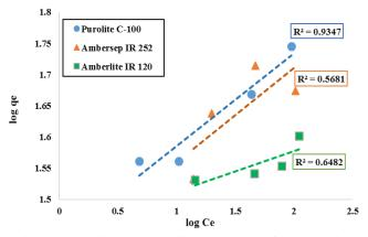
Fig. 13 The linear Freundlich isotherms for absorbing calcium ion using Purolite C-100 Na<sup>+</sup>, Ambersep IR 252 H<sup>+</sup>, and Amberlite IR 120 H<sup>+</sup> under the experimental condition of constant initial concentration, 60 min contact time, 350 rpm and  $25^{\circ}$ C
