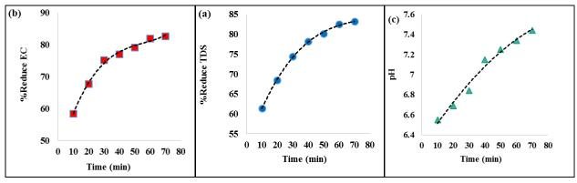
Fig. 19 The reduction of (a) TDS, (b) EC and (c) pH at optimum concentration, (3 g/L cationic resin and 12 g/L anionic resin)
