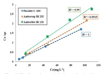
Fig. 12 The linear Langmuir isotherms for absorbing calcium ion using Purolite C-100 Na<sup>+</sup>, Ambersep IR 252 H<sup>+</sup>, and Amberlite IR 120 H<sup>+</sup> under the experimental condition of constant initial concentration, 60 min contact time, 350 rpm, and  $25^{\circ}$ C
