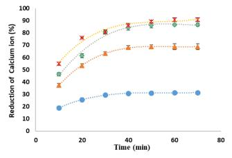
• 1 gr/L resin  $\triangleq$  2 gr/L resin  $\triangleq$  3 gr/L resin  $\cong$  4 gr/L resin Fig. 6 The reduction of calcium ion versus contact time using Ambersep IR252 H<sup>+</sup> at 25°C and 350 rpm.
