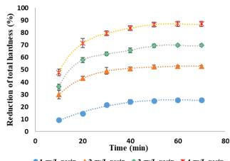
• 1 gr/L resin  $\blacktriangle$  2 gr/L resin  $\diamondsuit$  3 gr/L resin  $\divideontimes$  4 gr/L resin Fig. 8 The reduction of total hardness versus contact time using Amberlite IR120 H<sup>+</sup> at 25°C and 350 rpm.
