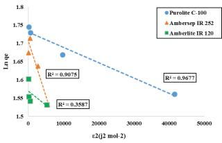
Fig. 15 The linear Dobinin-Radskvich isotherms for absorbing calcium ion using Purolite C-100 Na<sup>+</sup> Ambersep IR 252 H<sup>+</sup> and Amberlite IR 120 H<sup>+</sup> under the experimental condition of constant initial concentration, 60 min contact time, 350 rpm, and  $25^{\circ}$ C
