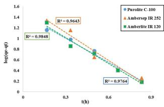
Fig. 16 The linear pseudo-first-order kinetic model for absorbing calcium ion using Purolite C-100 Na<sup>+</sup>, Ambersep IR 252 H<sup>+</sup> and Amberlite IR 120 H<sup>+</sup> under the experimental condition of constant initial concentration, 60 min contact time, 350 rpm, and  $25^{\circ}$ C
