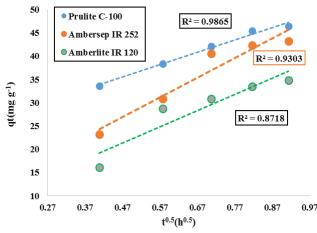
Fig. 18 The morris-Webber kinetic model for absorbing calcium ion using Purolite C-100 Na<sup>+</sup>, Ambersep IR 252 H<sup>+</sup> and Amberlite IR 120 H<sup>+</sup> under the experimental condition of constant initial concentration, 60 min contact time, 350 rpm, and  $25^{\circ}$ C
