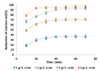
Fig. 3 The reduction of calcium ion versus contact time using Purolite C-100 Na<sup>+</sup> at 25°C and 350 rpm
