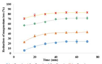
•1 gr/L resin  $\triangle 2$  gr/L resin  $\diamond 3$  gr/L resin  $\times 4$  gr/L resin Fig. 7 The reduction of magnesium ion versus contact time using Ambersep IR252 H<sup>+</sup> at 25°C and 350 rpm
