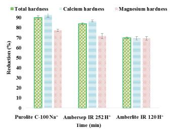
Fig. 11 The comparison of the removal percentage of total hardness, calcium ion and magnesium ion using strong cationic resins under optimum conditions
