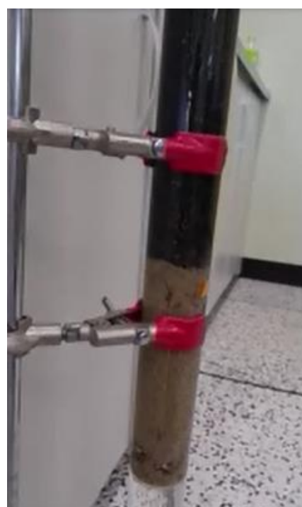
(b) Stratified layer formation using the dual media with sand B and anthracite B
