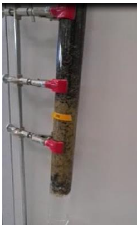
(a) Mixed layer formation using the dual media with sand A and anthracite A
