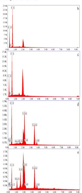
Fig. 7 EDS images of clean membrane and the membranes used in the study (a: Clean membrane, b:  $\Delta T$ = 20°C, v= 0.337 m/s and t = 6 hours, c:  $\Delta T$ = 50°C, v = 0.337 m/s and t = 6 hours, d:  $\Delta T$ = 40°C, v =0.73 m/s and t = 75 hours, e:  $\Delta T$ = 50°C, v =0.73 m/s and t = 50 hours)
