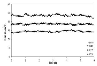
Fig. 3 Flux obtained for different feed circulation rates (at  $\Delta T = 50$ °C)
