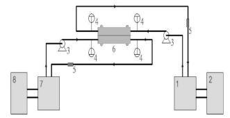
Fig. 1 MD Experiment Setup (1-Permeate Tank, 2-Cooling System, 3-Peristaltic Pump, 4-Thermocouples, 5-Conductivity and pH Measurement Probe, 6- Layer Membrane Module, 7-Feed Tank, 8-Water Circulator)
