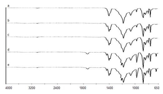
Fig. 8 FT-IR analysis (a) Clean membrane, (b)  $\Delta T = 20^{\circ}$ C, v = 0.337 m/s and t = 6 hours, (c)  $\Delta T = 50^{\circ}$ C, v = 0.337 m/s and t = 6 hours, (d)  $\Delta T = 50^{\circ}$ C, v = 0.73 m/s and t = 50 hours, (e)  $\Delta T = 40^{\circ}$ C, v = 0.73 m/s and t = 75 hours
