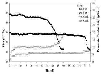
Fig. 5 Long term operational flux graph for  $\Delta T = 40^{\circ}$ C and  $\Delta T = 50^{\circ}$ C
