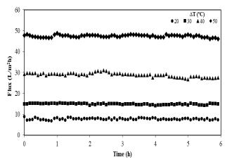
Fig. 2 Flux obtained for different  $\Delta T$  (v = 0.73 m/s)
