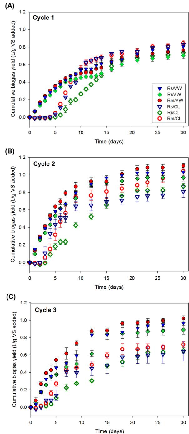
Fig. 1 Cumulative biogas yield during subcultures. Curves are labeled with the corresponding inoculum sources and substrates (CL, cellulose)
