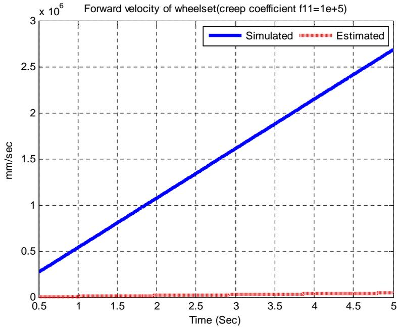
Fig. 4 Forward velocity wheelset at creep co-efficient 1e+5
