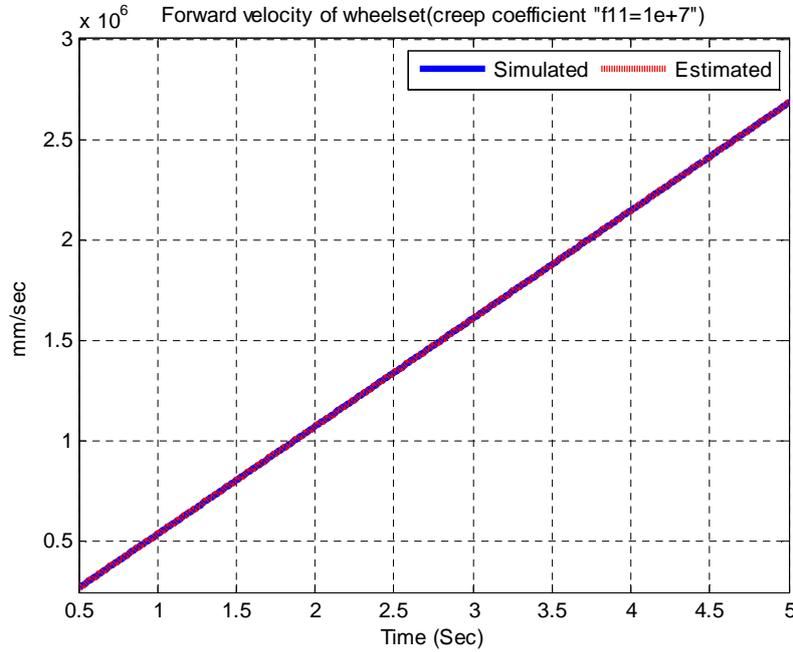
Fig. 2 Forward velocity wheelset at creep co-efficient of  $10^7$
