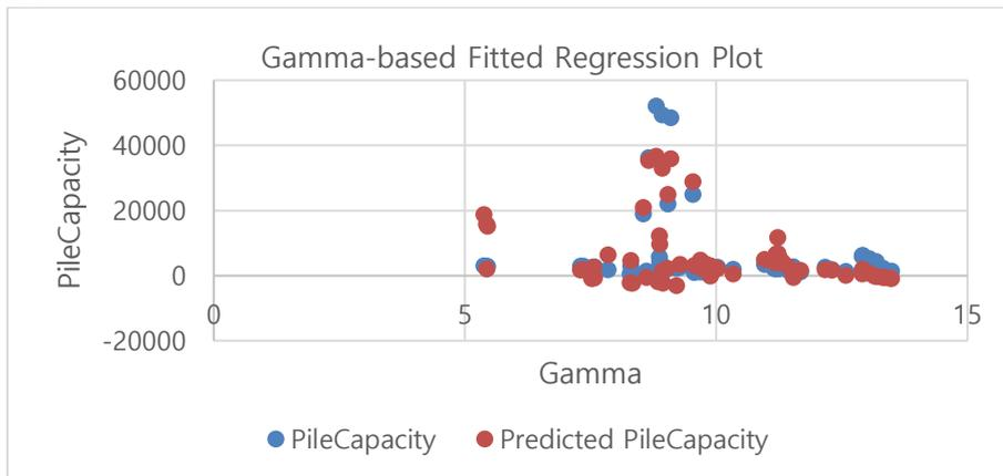
(c) Regression plot of measured vs. predicted pile bearing capacity for effective soil specific weight (Gamma) variable
