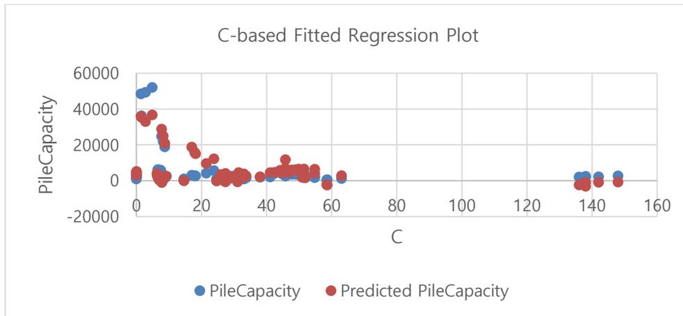
(a) Regression plot of measured vs. predicted pile bearing capacity for drained soil cohesion (C) variable
