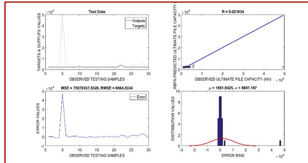
Fig. 5 Resulted charts for testing datasets associated with fitting curve, R, MSE, RMSE and error histogram parameters
