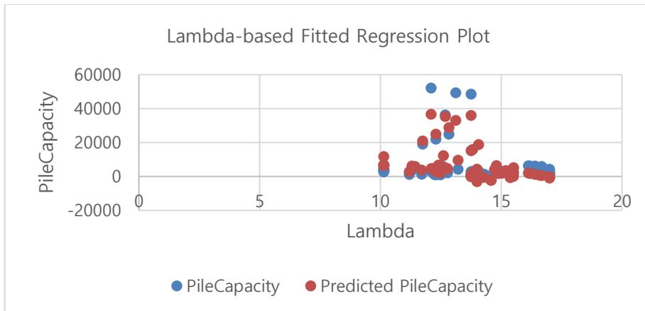
(d) Regression plot of measured vs. predicted pile bearing capacity for pile-soil interface friction angle (Lambda) variable
