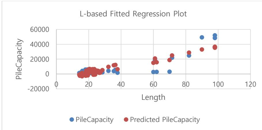
(g) Regression plot of measured vs. predicted pile bearing capacity for embedded pile length (L) variable
