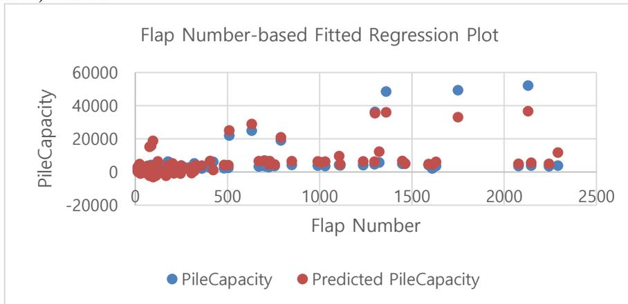
(e) Regression plot of measured vs. predicted pile bearing capacity for hammer strikes (Flap Number) variable
