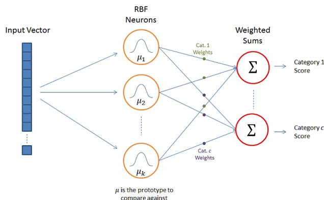
Fig. 1 RBF type neural network structure
