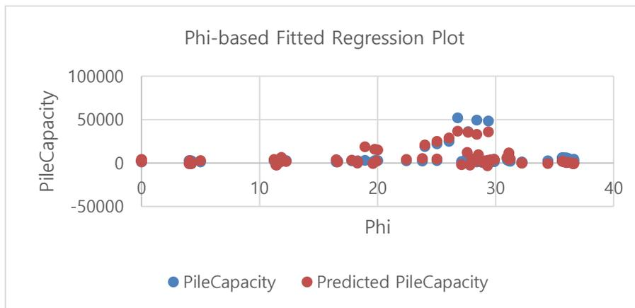
(b) Regression plot of measured vs. predicted pile bearing capacity for drained soil friction angle (Phi) variable
