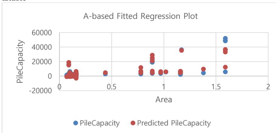
(f) Regression plot of measured vs. predicted pile bearing capacity for pile cross section area (A) variable
