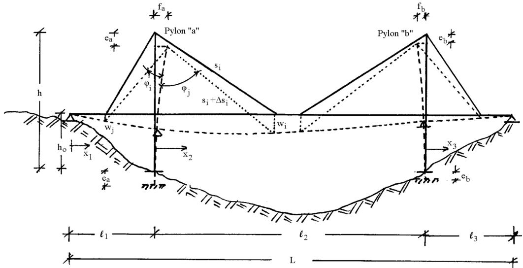
Fig. 2 Relative displacement of two neighboring pylons due to a fault movement
