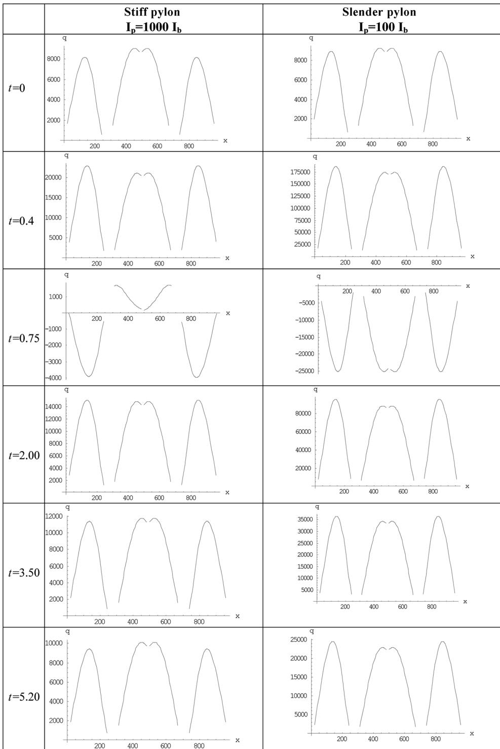
Fig. 17 The tensions of the cables at various time instants
