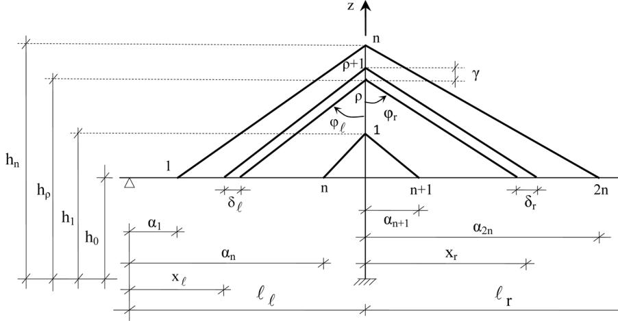
Fig. 8 Harp system of cables with dense arrangement
