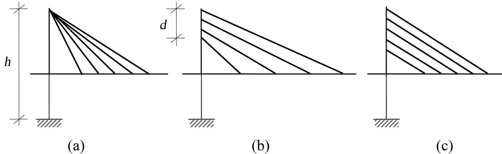
Fig. 1 Cable layout: (a) Fan system, (b) Harp system and (c) Parallel system of cables
