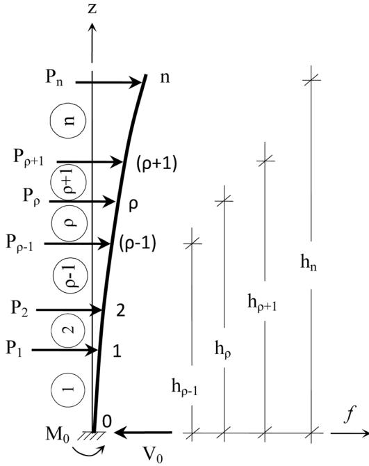
Fig. 7 Pylon stressing due to cables
