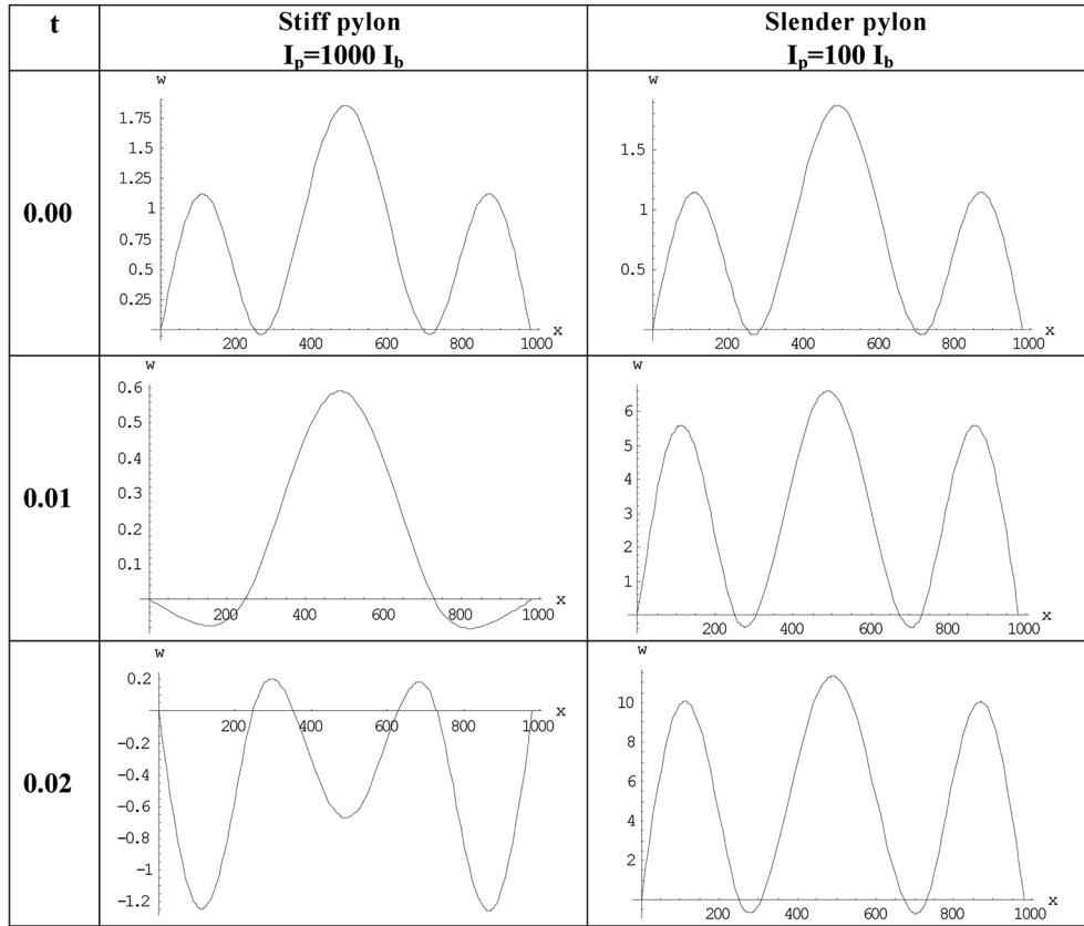
Fig. 18 Deformations of the bridge-deck
