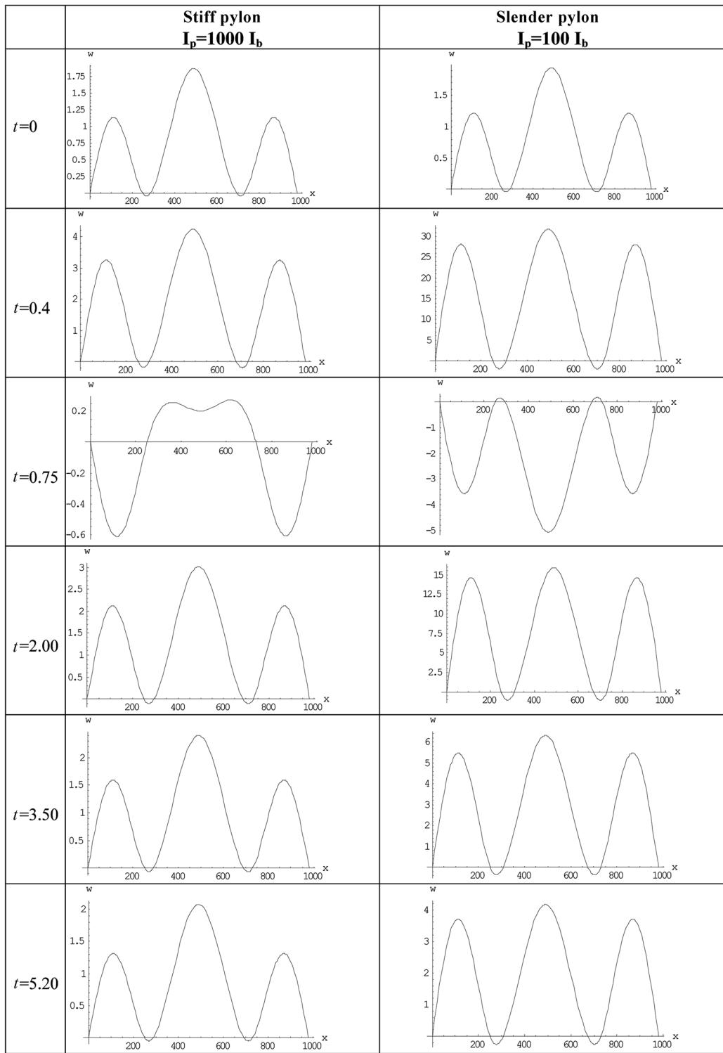
Fig. 16 The deformed shape of the bridge deck at different instants of the pylons' movement
