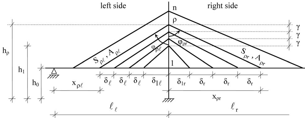
Fig. 6 Cable arrangement in a harp system
