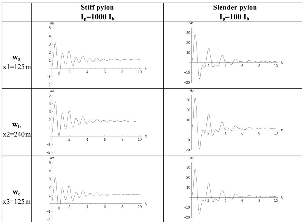
Fig. 15 Dynamic displacements at midspan for stiff and slender pylons
