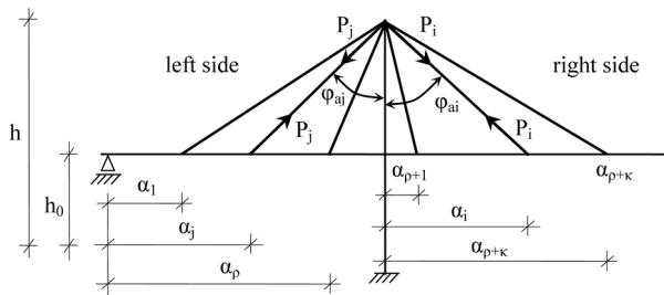
Fig. 4 Forces acting on the pylon due to the cables
