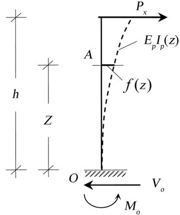
Fig. 3 Deformed configuration of the pylon
