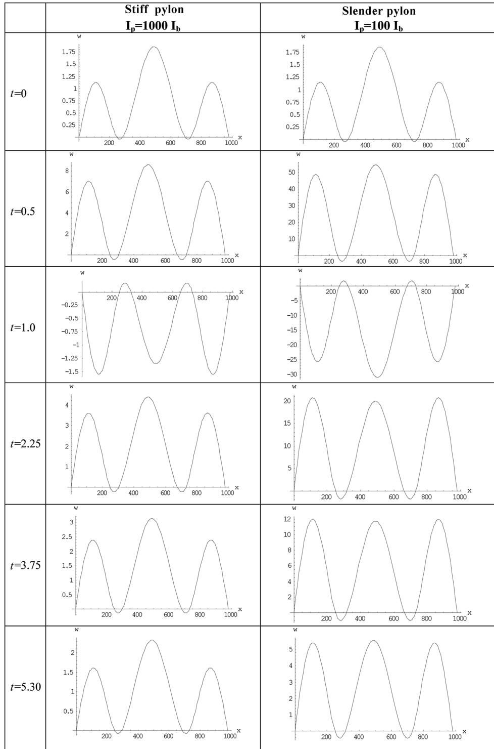
Fig. 12 The deformed shape of the bridge deck at different instants of the pylons' movement
