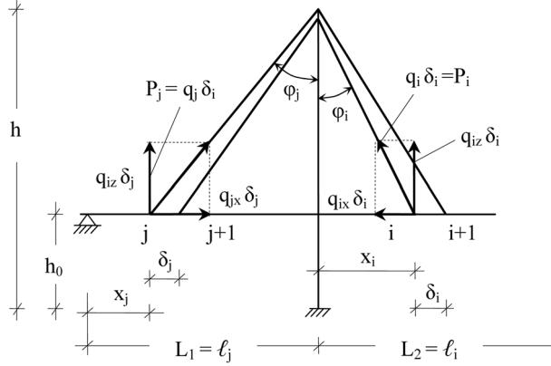
Fig. 5 Pylon force equilibrium under a dense arrangement of cables
