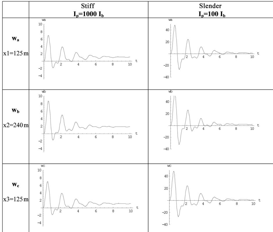
Fig. 11 Dynamic displacements at midspan for stiff and slender pylons
