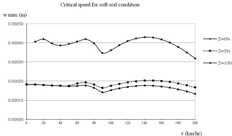
Fig. 2 Maximum dynamic deflection response spectra as a function of velocity for various values of damping ratio for  $P_0 = 80$  kN,  $\omega_{beb} = 100$  rad/sec,  $acc = 2$  m/sec $^2$ ,  $\zeta = 5\%, 10\%$
