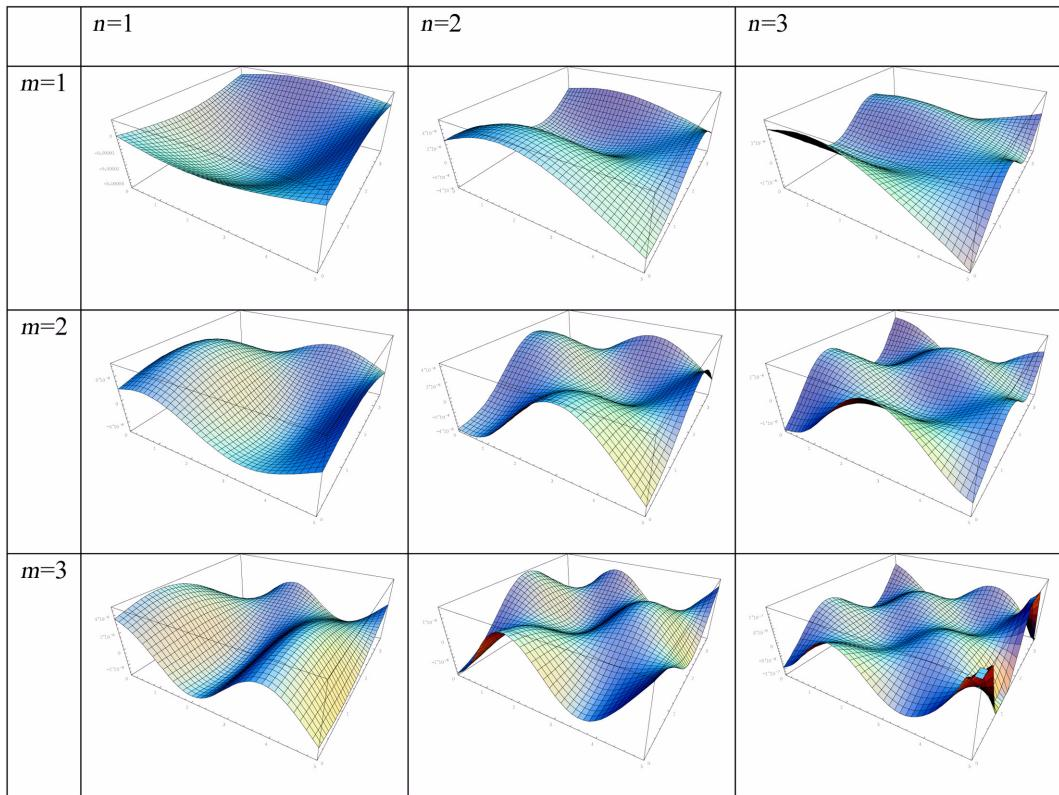
Fig. 5 The dynamic deflection distribution over the plate region to the moving dynamic traffic load calculated at  $x = a/2$  and  $y = b/2$  during the interval  $0 \leq t \leq t_0$ ,  $P_0 = 80$  kN,  $v = 90$  km/hr,  $acc = 2$  m/sec $^2$ ,  $\omega_{load} = 100$  rad/sec,  $t = 0.0996$  sec,  $\zeta = 5\%$
