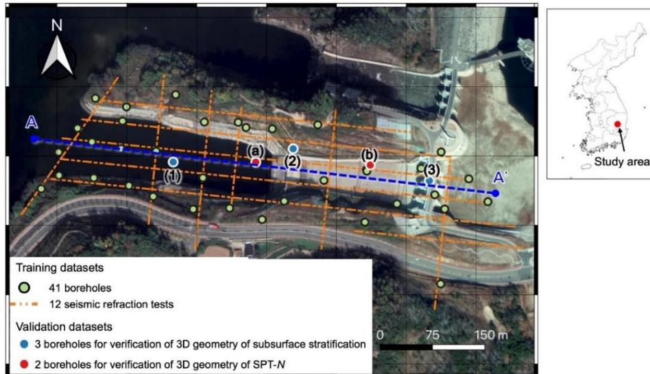
Fig. 1 Plan view of the borehole location and seismic refraction test lines at a dam-emergency-spillway construction site in Gyeongsangbuk-do, South Korea
