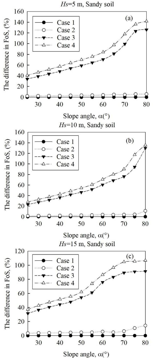
Fig. 8 The difference in FoS for sandy soil slope, (a)  $H_s$  is 5 m, (b)  $H_s$  is 10 m and (c)  $H_s$  is 15 m
