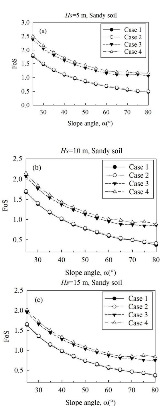
Fig. 5 FoS for sandy soil slopes, (a)  $H_s$  is 5 m, (b)  $H_s$  is 10 m and (c)  $H_s$  is 15 m
