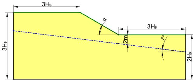
Fig. 2 Illustration of the geometry of the typical slope
