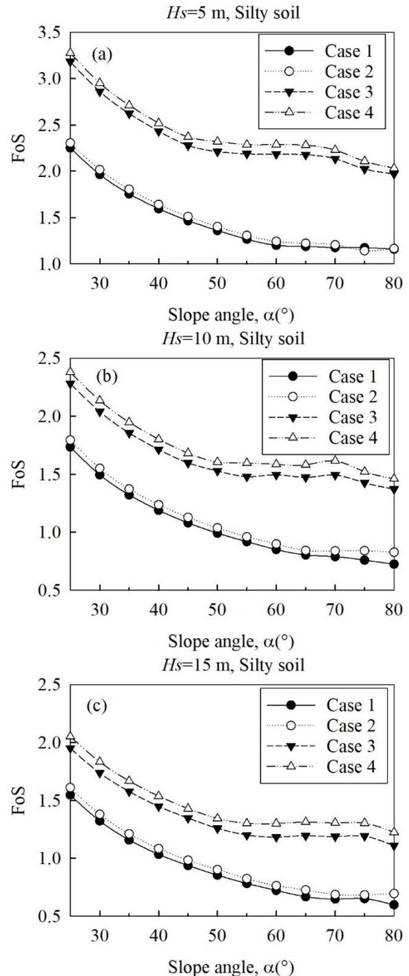
Fig. 6 FoS for silty soil slope, (a)  $H_s$  is 5 m, (b)  $H_s$  is 10 m and (c)  $H_s$  is 15 m
