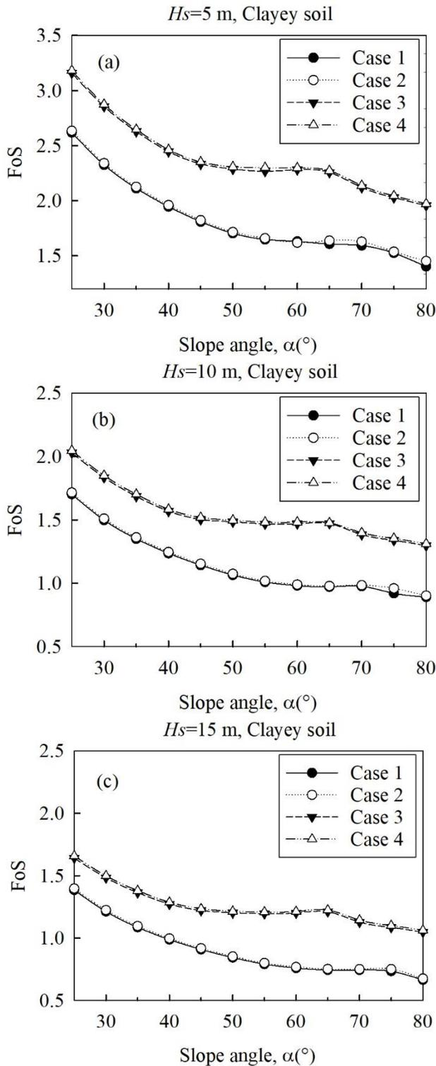
Fig. 7 FoS for clayey soil slope, (a)  $H_s$  is 5 m, (b)  $H_s$  is 10 m and (c)  $H_s$  is 15 m
