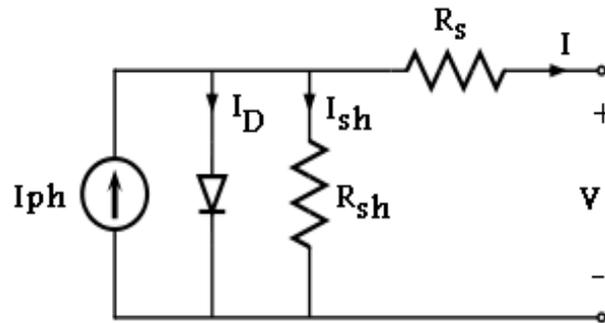
Fig. 2 PV cell equivalent circuit
