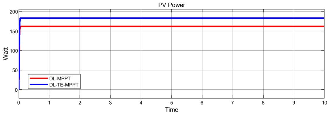
Fig. 11 DL-MPPT PV System Power with and Without Coolant
