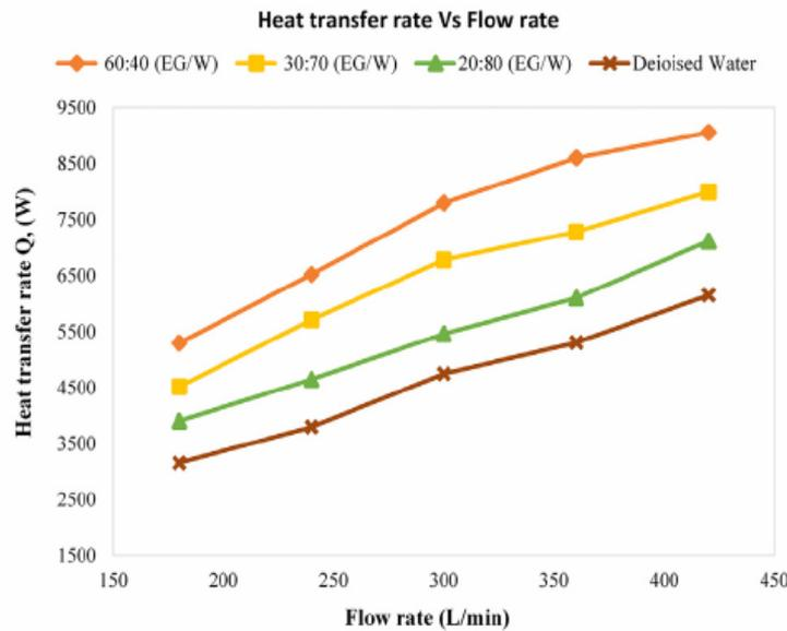
Fig. 8 Heat transfer rate characteristics (Shankara *et al.* 2022)
