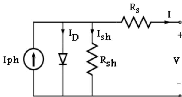
Fig. 2 PV cell equivalent circuit
