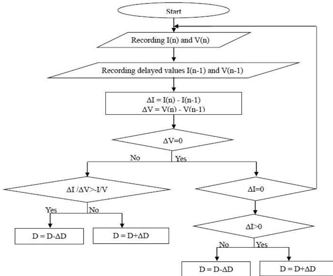
Fig. 5 Incremental conductance MPPT flow chart
