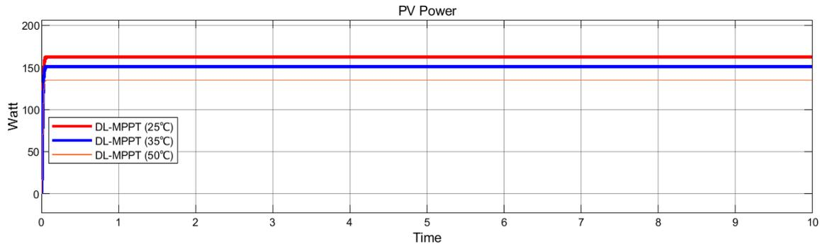
Fig. 12 Comparison of DL-MPPT power at variable temperature
