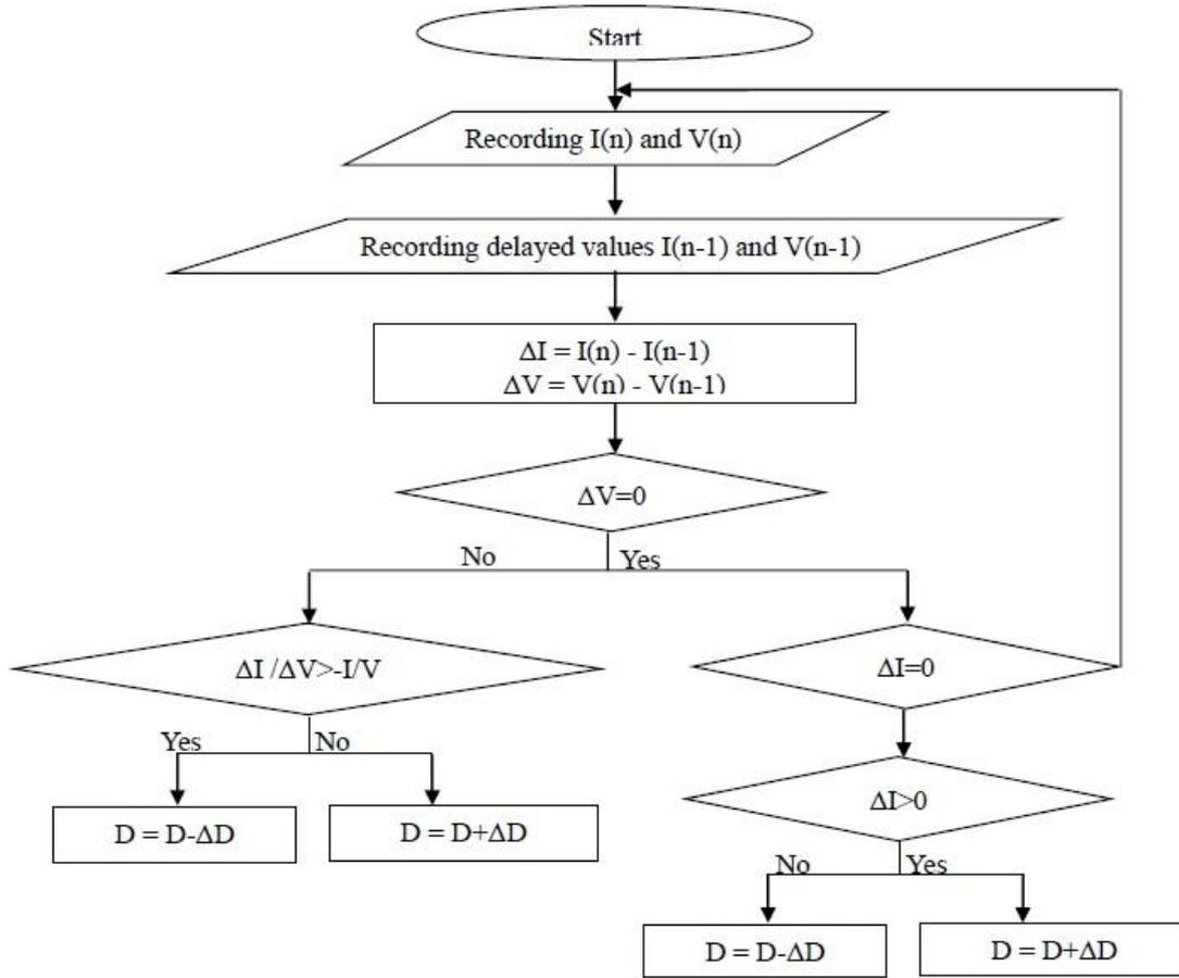
Fig. 5 Incremental conductance MPPT flow chart
