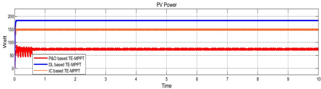
Fig. 14 Comparison of different MPPT algorithm output
