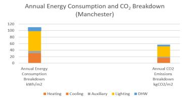
Fig. 9 Annual energy consumption and CO<sub>2</sub> breakdown
