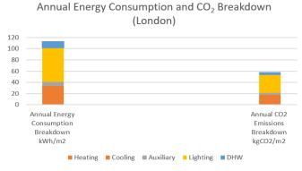
Fig. 6 Annual Energy Consumption and CO2 breakdown
