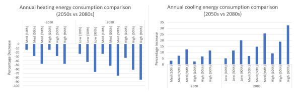
Fig. 8 (a) Annual heating energy consumption (2050s vs 2080s); (b) Annual cooling energy consumption (2050s vs 2080s)
