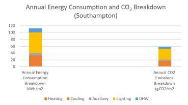
Fig. 12 Annual energy consumption and  $CO_2$  breakdown
