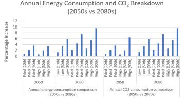
Fig. 7 Annual energy and CO<sub>2</sub> consumption comparison (2050s vs 2080s)
