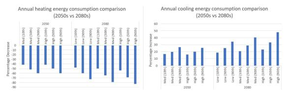
Fig. 14 (a) Annual heating energy consumption (2050s vs 2080s); (b) Annual cooling energy consumption (2050s vs 2080s)
