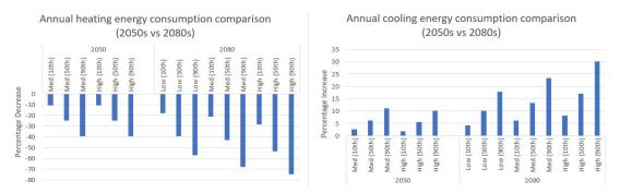
Fig. 11 (a) Annual heating energy consumption (2050s vs 2080s); (b) Annual cooling energy consumption (2050s vs 2080s)
