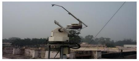
Fig. 1 Pictorial view of measuring system used which records the solar radiation
