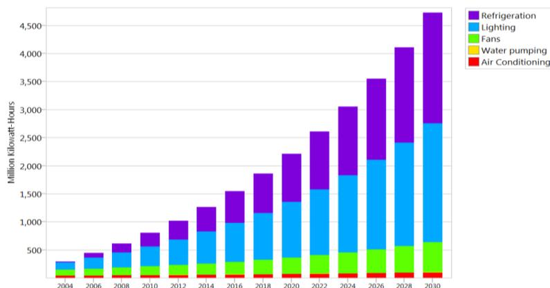
Fig. 3.1 Projection of urban demand for electricity developed by LEAP model
