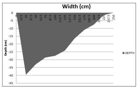
Fig. 5 Depth of the Rivulet across its width
