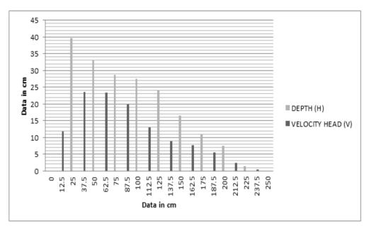
Fig. 7 Combined distribution of depth and velocity distribution across the width of the Rivulet
