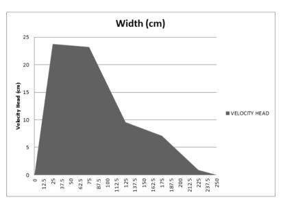
Fig. 6 Velocity distribution across the width of the Rivulet
