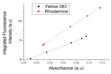
Fig. 7 Integrated fluorescence intensity for Lumogen Yellow 083 and reference Rhodamine dye
