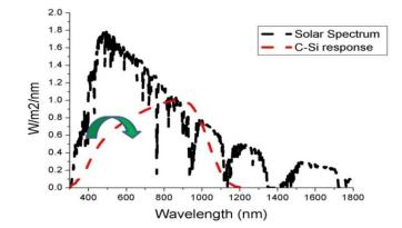
Fig. 1 Luminescent down-shifting process to increase solar cell active range and efficiency. High energy photons are re-radiated at a longer wavelength, better matching the photosensitivity spectral response of the c-Si solar cell
