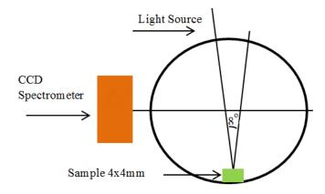
Fig. 8 Schematic diagram of integrated sphere setup for LQY measurements
