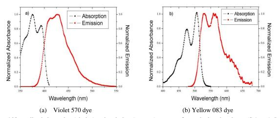
Fig. 4 Normalized absorption (circles) and emission (squares) spectra of organic dyes in toluene (0.1 mg/ml)
