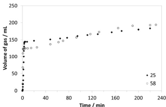
Fig. 2 Evolution of  $H_2 + N_2$  as a function of time for 25 and 58 at  $50^\circ C$
