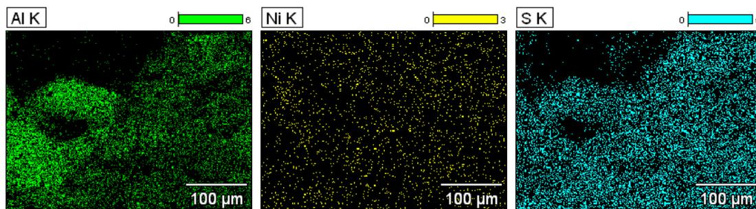
Fig. 3. Mapping of 58 by EDX: distribution of Ni, Ti and S.
