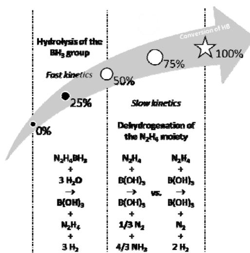
Fig. 1 Dehydrogenation of hydrazine borane  $N_2H_4BH_3$ , a two-step process
