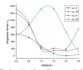
Fig. 4 variation of tangential stress  $\sigma_{zr}$  with the distance *r* (concentrated normal force)
