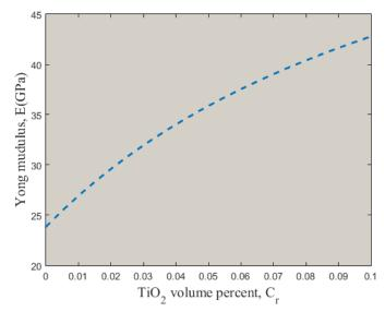
Fig. 1 The effect of TiO<sub>2</sub> nanoparticles on the elastic modulus of the concrete
