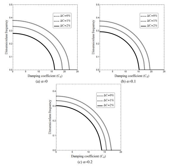
Fig. 3 Normalized frequency of FG nanoplate according to damping coefficient for diverse pore volume fraction (p=1, a/h=10,  $\Delta T=10$ ,  $K_w=5$ ,  $K_p=0.5$ ,  $\mu=0.2$ ,  $\lambda=0.1$ )
