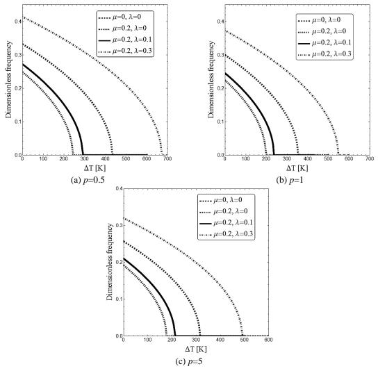
Fig. 2 Changing of normalized frequency for ideal nanoplates with respect to temperature variation based on diverse nonlocality and strain gradients factors (a/h=15,  $K_w=0$ ,  $K_p=0$ ,  $\Delta C=0\%$ )
