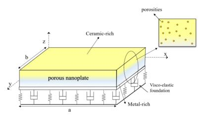
Fig. 1 Geometry of porous FG composite nanoplate coupled by visco-elastic medium
