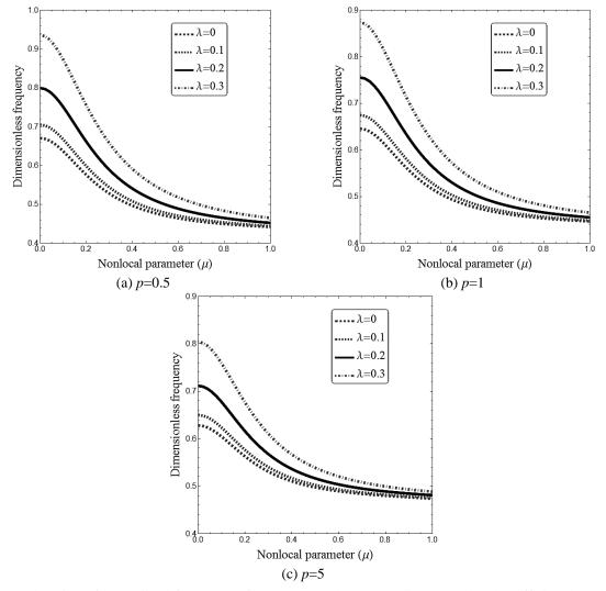
Fig. 4 Changing of normalized frequency of porous nanoplates according to nonlocal coefficient based on diverse strain gradients coefficient ( $\Delta T$ =50,  $\Delta C$ =1%, a/h=10,  $K_w$ =25,  $K_p$ =10)
