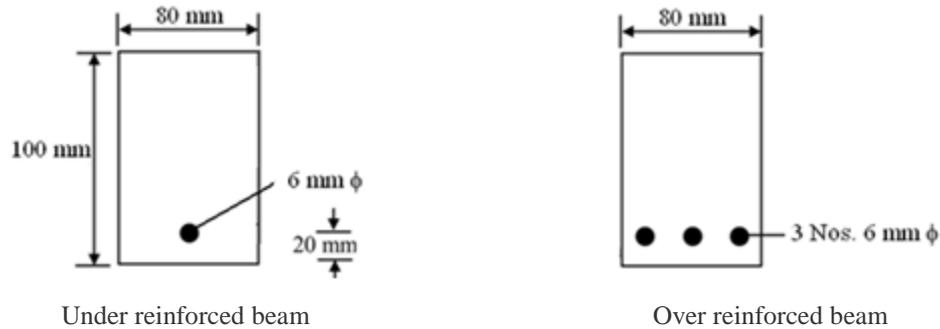
Fig. 3 Reinforcement details for the beams
