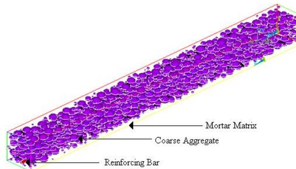
Fig. 2 Concrete mesostructure with reinforcing bar
