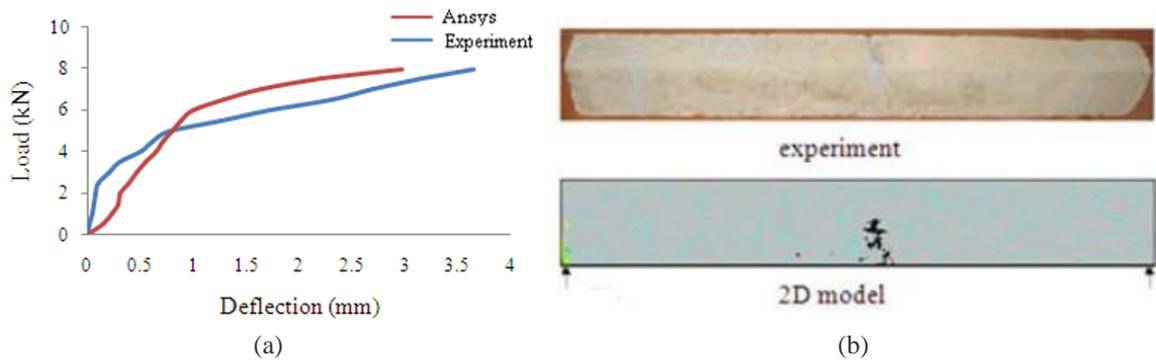
Fig. 5 (a) Load-deflection plot at mid-span and (b) crack Pattern of the beam-II
