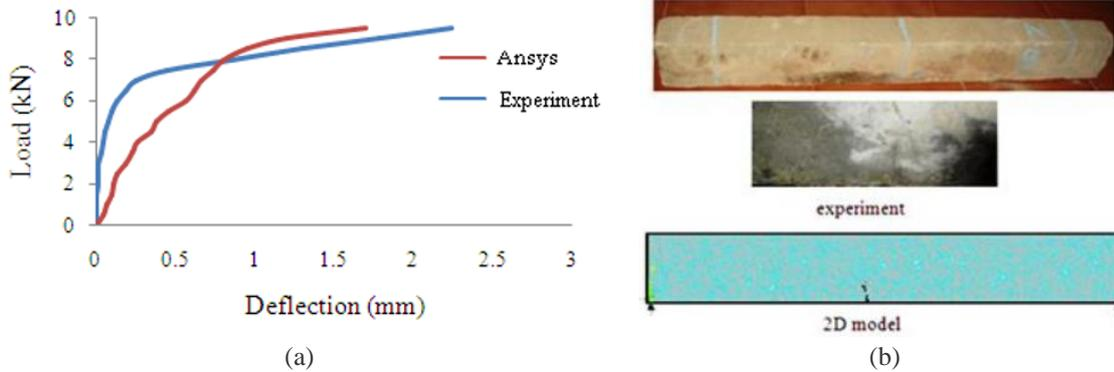
Fig. 7 (a) Load-deflection plot at mid-span and (b) crack Pattern of the beam-VI
