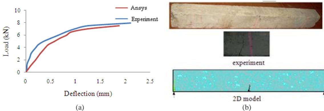
Fig. 6 (a) Load-deflection plot at mid-span and (b) crack Pattern of the beam-III
