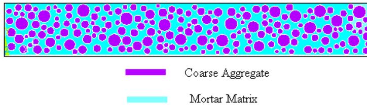
Fig. 1 2D Concrete mesostructure
