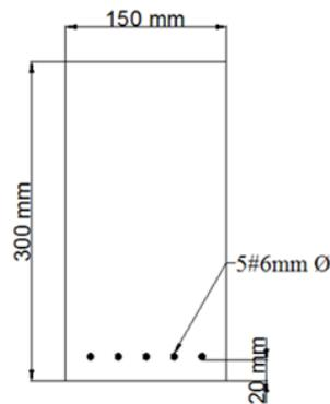
Fig. 4 Reinforcement details for the beams
