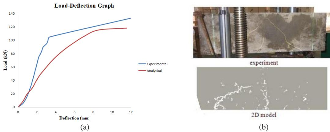
Fig. 8 (a) Load-deflection plot at mid-span and (b) crack Pattern of the deep beam
