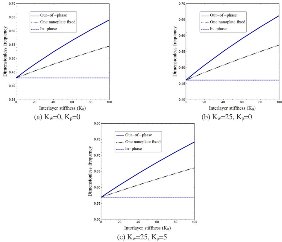
Fig. 5 Normalized frequency of double-coupled nanoplate against interlayer stiffness for various elastic foundation parameters ( $a/h=10$ ,  $e_0=0.5$ ,  $\mu=0.2$ ,  $\Delta T=0.1$ ,  $\lambda=0.1$ )
