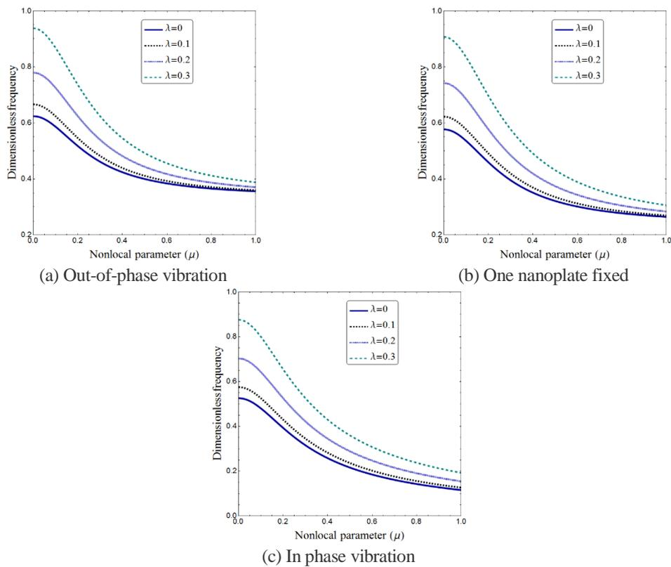
Fig. 3 Normalized frequency of double-coupled nanoplate against nonlocal and strain gradient parameters ( $a/h=10, K_w=0, K_p=0, \Delta T=0, K_0=50, e_0=0.5$ )
