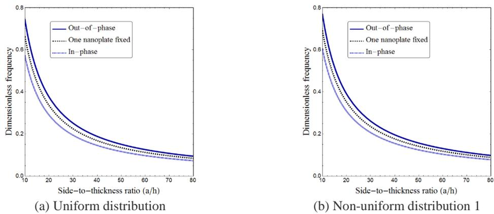
Fig. 6 Normalized frequency of double-coupled nanoplate against side-to-thickness ratio for different types of vibration ( $e_0=0.5$ ,  $K_w=25$ ,  $K_p=5$ ,  $\mu=0.2$ ,  $\Delta T=0.1$ ,  $K_0=100$ )
