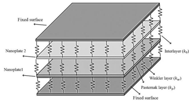
Fig. 2 A double-coupled nanoplate system
