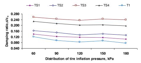
Fig. 6 The vertical equivalent damping ratios of T1, TS1, TS2, TS3 and TS4 test in soil depth of 80 mm
