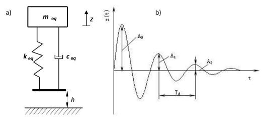
Fig. 2(a) Single degree of freedom system for measuring the vertical equivalent damping ratio of tire and tire-soil system; (b) The decay curve of the free vibration with damping
