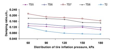
Fig. 8 The vertical equivalent damping ratio of T2, TS5, TS6, TS7 and TS8 tests in soil depth of 80 mm
