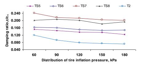
Fig. 9 The vertical equivalent damping ratio of T2, TS5, TS6, TS7 and TS8 tests in soil depth of 120 mm
