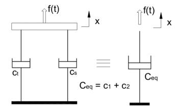
Fig. 10 New damping model of tire-soil system  $c_{eq}$  - equivalent damping coefficient of tire-soil system;  $c_t$  - damping coefficient of tire;  $c_s$  - damping coefficient of paddy soil
