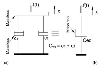
Fig. 5(a) A parallel combination of massless dampers; (b) Equivalent system with only one damper for a parallel combination (Taylor 2000)
